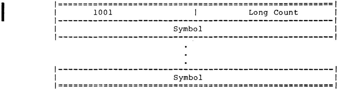
Block type 1001 is used to declare symbolic entry points. Each word contains one SIXBIT symbol. This block is similar in function to block type 4.
