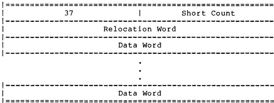
Block Type 37 contains a debugging symbol table for COBDDT, the COBOL debugging program. If local symbols are being loaded, the table is loaded.
