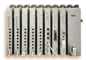
The DEChub 90 workgroup chassis is the industry's only stackable and hub-based solution in one product. It is designed to support the communication needs of today's workgroups in small to mid-sized companies, and expanding communication needs in corporate enterprise networks.
