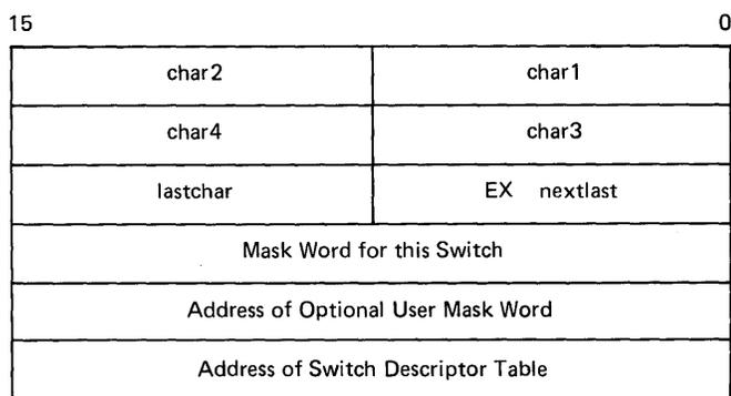
Figure 6-2 Format of Switch Descriptor Table Entry
