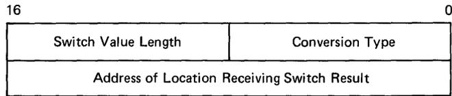
Figure 6-3 Format of Switch-Value Descriptor Table Entry
