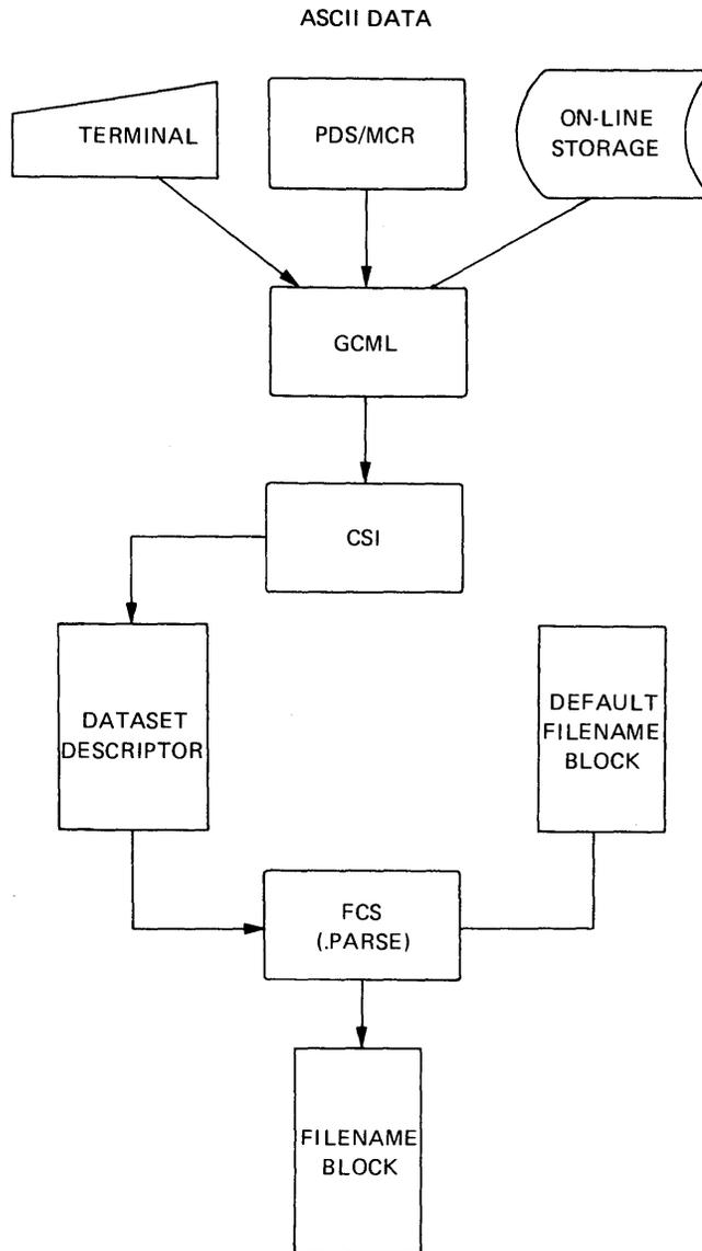
Figure 6-1 Data Flow During Command Line Processing
