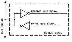
Figure 8-1 Bidirectional Nature of the Bus
