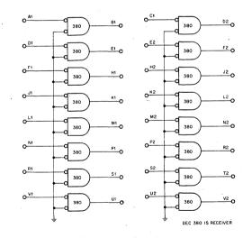
Figure 9.4 M784 Unibus Receivers
