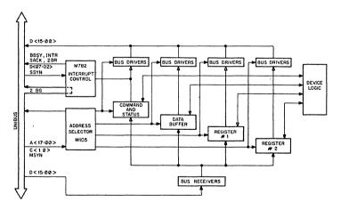
Figure 9.1 Typical Peripheral Device Interface
