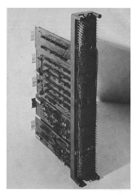
All PDP-11 processors, memories and peripherals are electrically and mechanically modular subsystems supported in System Units which are simply plugged together to form a computer tailored to user needs.
