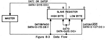
Note that all transfers into the master are word operations; it is up to the master to accept the appropriate byte. On a DATOB, the master must place the byte on the appropriate data lines; the slave must accept the proper byte.
