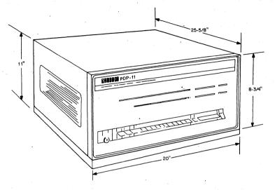
Figure 10.2 Table Top PDP-11 Dimensions
