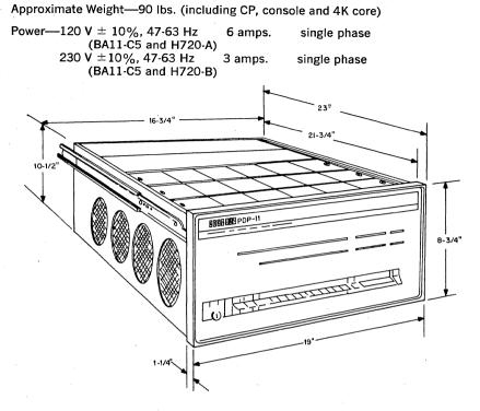
Figure 10.3 Rack Mountable PDP-11 Dimensions
