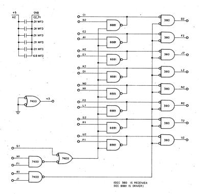
Figure 9.5 M785 Unibus Drivers and Receivers
