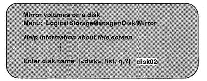
3. Select the target disk name (this disk must be the same size or larger than the originating disk). Volumes can be mirrored onto another disk or onto any available disk space.
