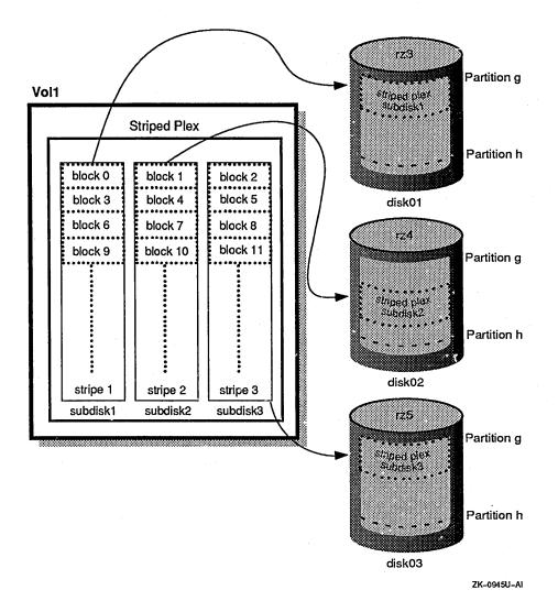
Figure 2-2: Striping Disks with the Logical Storage Manager
