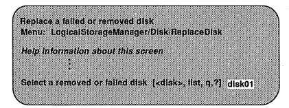
3. If there are any initialized disks available that are not part of a disk group, LSM displays the following screen to list the disks available to be used as a replacement. Select the replacement disk from the list provided.
