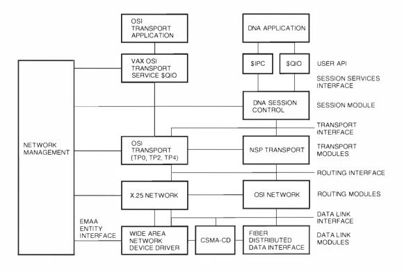
Figure 1 DECnet/OSI for OpenVMS Base Components
