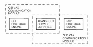
Figure 5 Logical Transport Components
