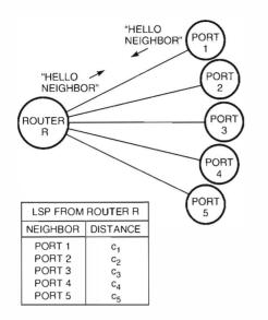
Figure 2 Link State Routing
