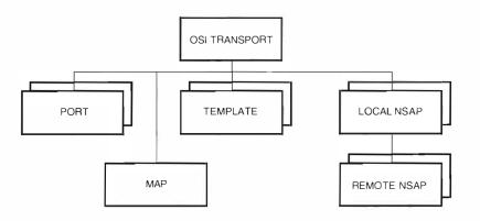
*Figure 6 Containment Hierarchy for OSI Transport Module*
