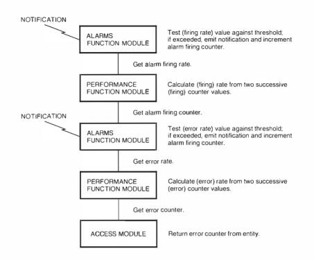
Figure 3 Data/Control Flow for Multiple FMs
