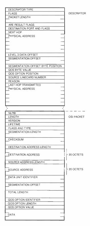
Figure 9 OSI Packet Buffer and Descriptor
