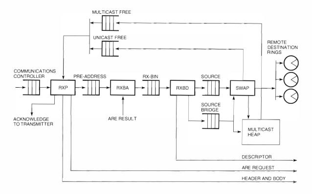
Figure 8 Linecard Receive Processing
