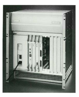
Figure 2 DECNIS 600 Backbone Router
