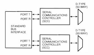
Figure 5 DEC WANcontroller 622 Block Diagram
