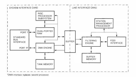
Figure 6 DEC FDDIcontroller 621 Block Diagram
