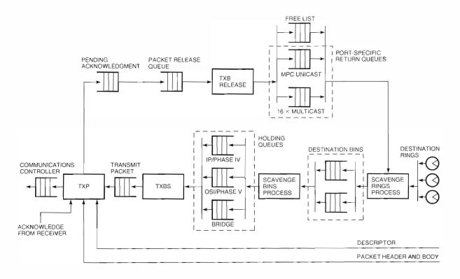
Figure 10 Linecard Transmit Processes
