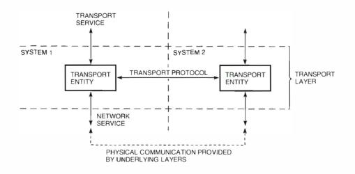
Figure 1 Elements of a Layer of DECnet Architecture
