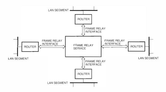
Figure 1 Typical Frame Relay Configuration
