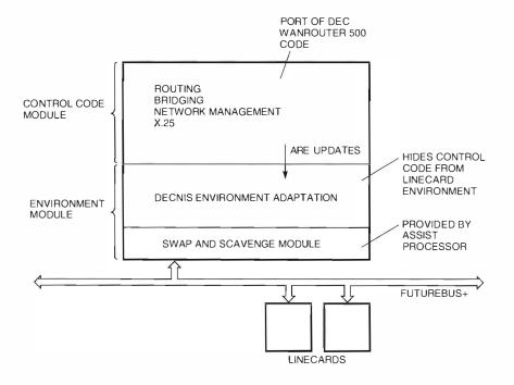
Figure 7 MPC Software Structure
