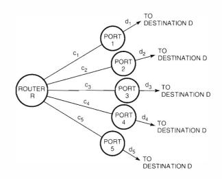
Figure 1 Distance Vector Routing
