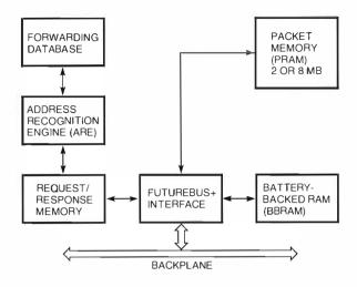
Figure 4 PRAM and ARE Module Block Diagram
