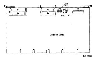
Figure 1-2B Diagnostic LED Locations on the UDA50 Modules
