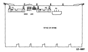
Figure 1-2A Diagnostic LED Locations on the UDA50 Modules
