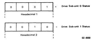
Figure 2-4 Sub-unit Mask Bit Layout Examples
