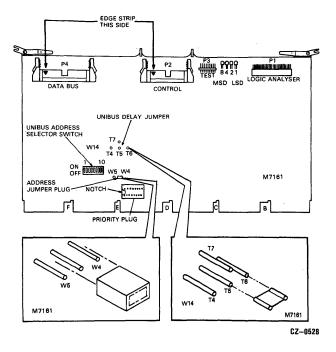
Figure 1-3A M7161 Address Switch and Jumper Locations
