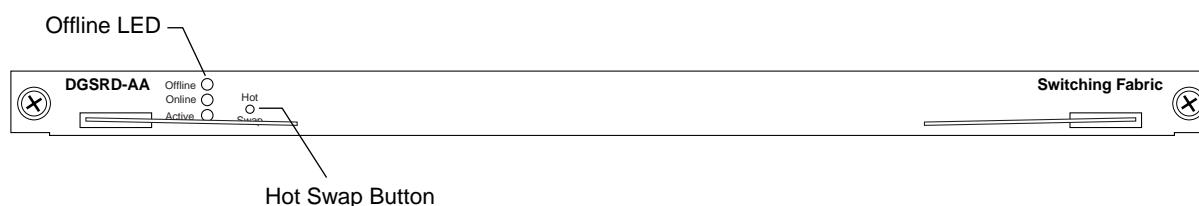
Figure 3. Location of Offline LED and Hot Swap button on a Switching Fabric Module
