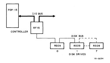
Figure 2-1 DECdisk System Configuration
