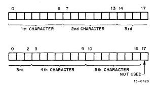
Figure 5-2 5/7 ASCII Packing Scheme
