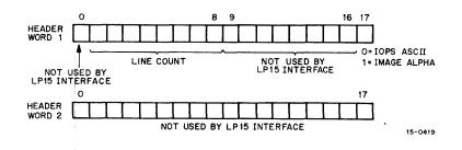
Figure 5-1 Data Buffer Header Format
