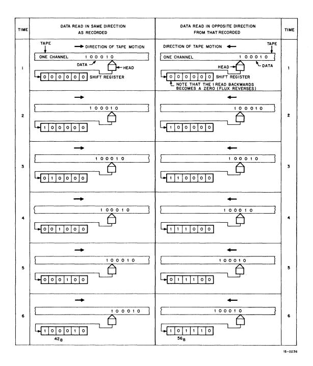
Figure 3–3 Bidirectional Reading and Writing
