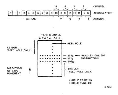
Figure 1-1 Tape Format and Accumulator Bits (Alphanumeric Mode)
