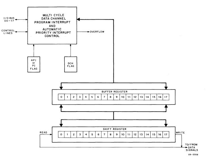
Figure 2-4 DECdisk Data Transfer Section
