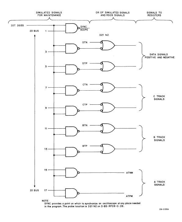
Figure 2-6 Simulating the RS09 with the Maintenance Logic
