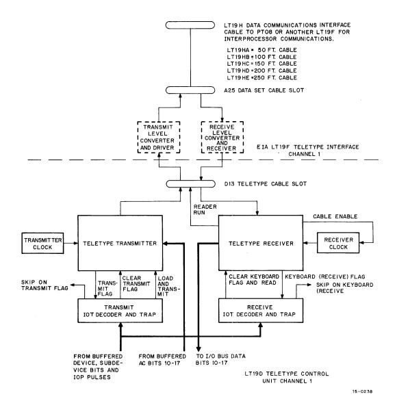
Figure 4-2 LT19E, F, H Teletype Control Interface & Communications
