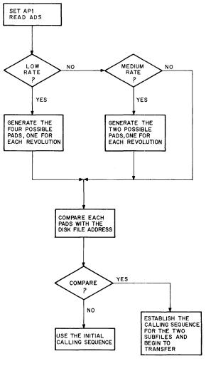
Figure 2–13 Flow Diagram of the Subroutine That Uses the ADS Register
