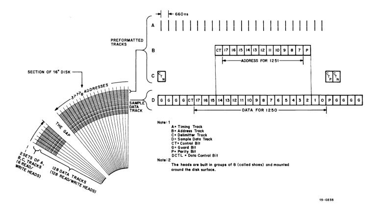
Figure 2-2 Disk Surface Recording Format
