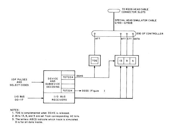
Figure 2-5 Simulating the Disk Surface with the Maintenance Logic
