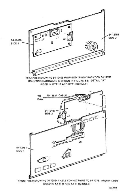
Figure 6-11 54-12498 Integral Modem Mounting and Cabling
