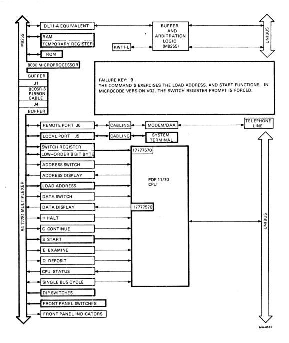
Figure 7-9 Failure Key 9
