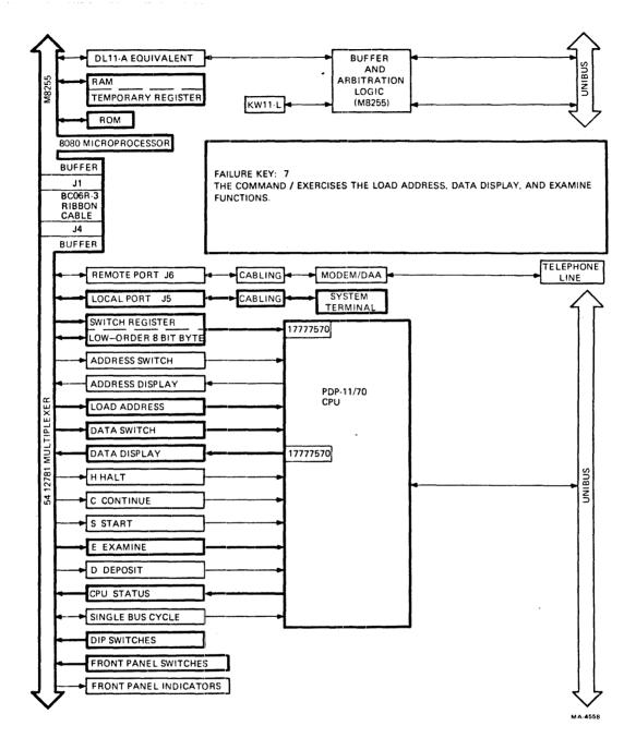
Figure 7-7 Failure Key 7
