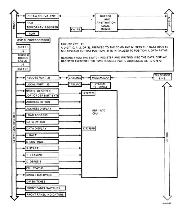
Figure 7-11 Failure Key 11
