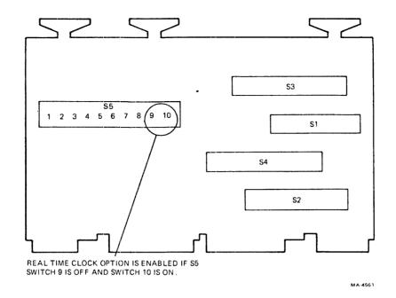
Figure 6-4 M7856 Switch Layout
