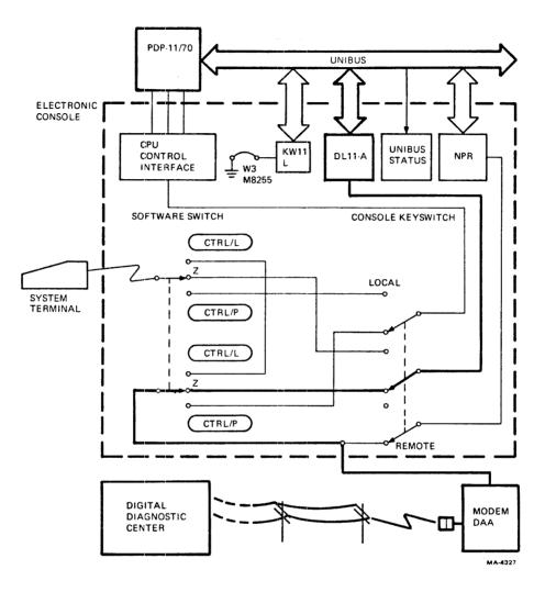
Figure 3-5 Remote Program I/O State
