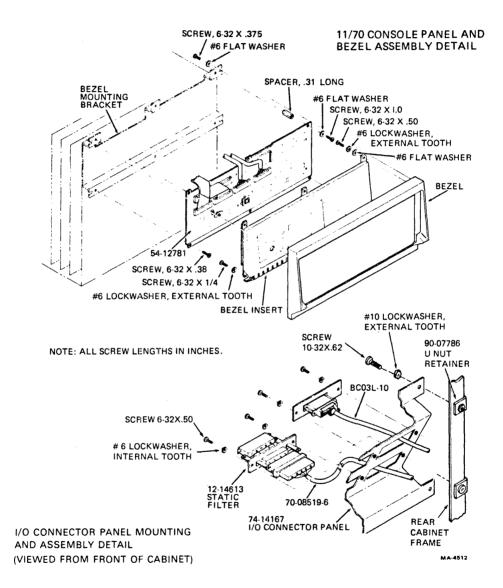
Figure 6-9 KY11-RB/KY11-RE Mechanical Assembly
