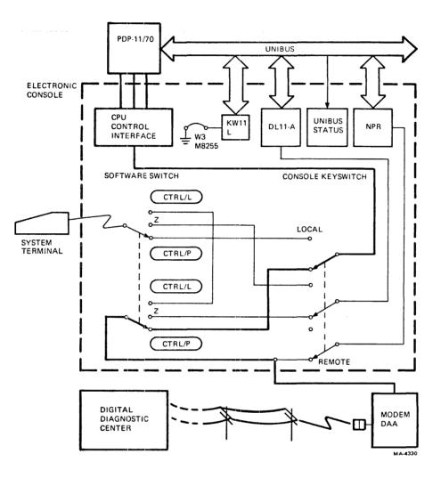
Figure 3-3 Remote Console State
