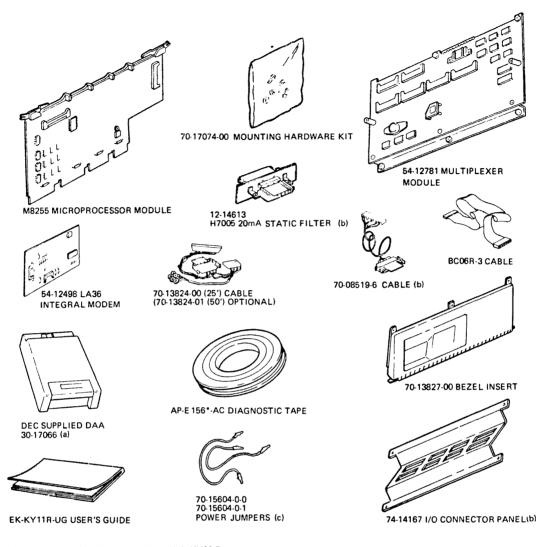
(a) SUPPLIED BY TELEPHONE COMPANY IN KY11-R (b) SUPPLIED BY BRANCH OFFICE IF NOT IN KIT (c) INCLUDED IN 70-17074 MOUNTING HARDWARE KIT
