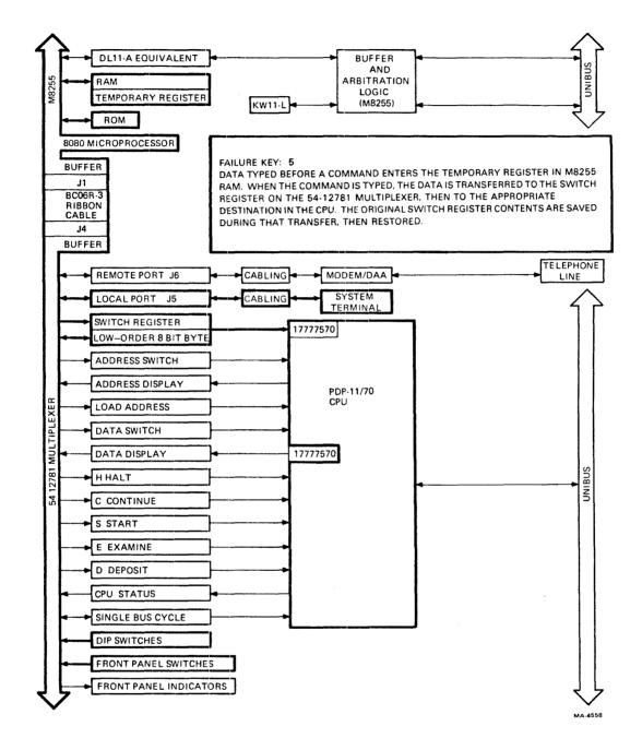
Figure 7-5 Failure Key 5
