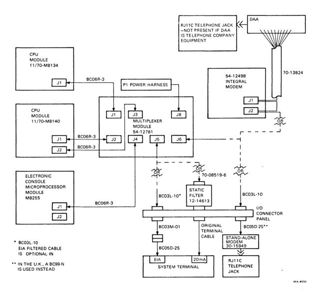
Figure 6-10 KY11-R Cabling Diagram
