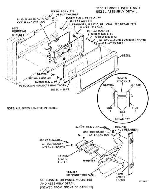
Figure 6-8 KY11-R/KY11-RC Mechanical Assembly
