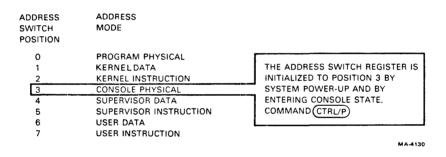
Figure 4-3 Address Display Multiplexer
