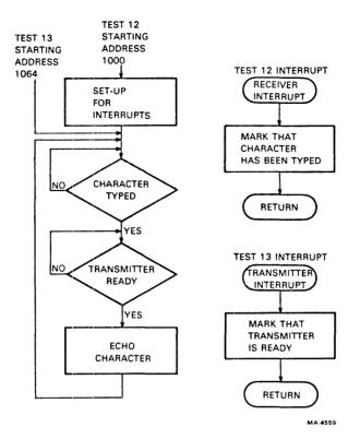
Figure 6-14 Flow Diagram (Tests 12 and 13)
