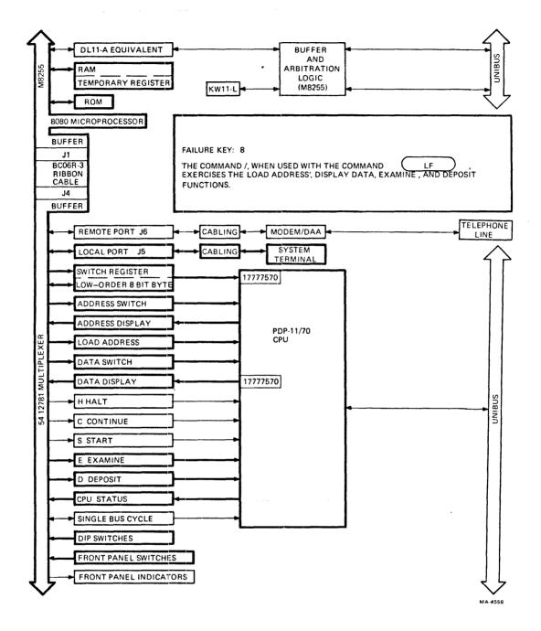
Figure 7-8 Failure Key 8
