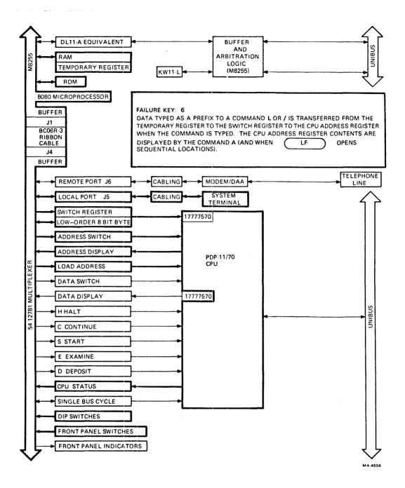
Figure 7-6 Failure Key 6
