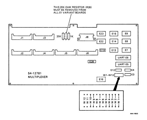
Figure 6-7 54-12781 Jumper Configuration and Layout
