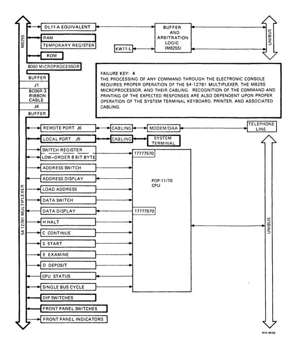
Figure 7-4 Failure Key 4
