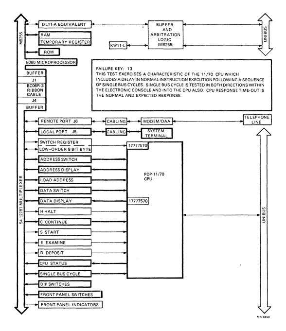
Figure 7-13 Failure Key 13
