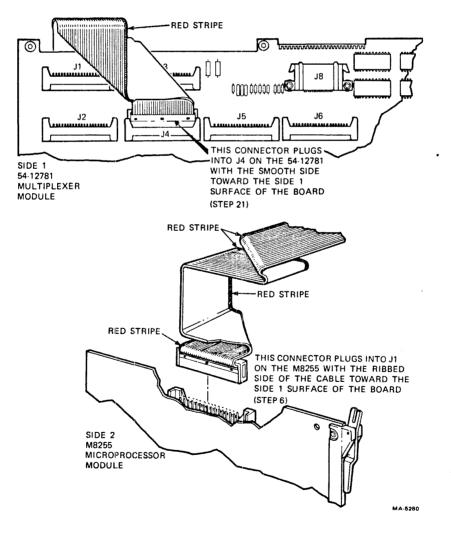
Figure 6-6 BC06R-3 Cable Configuration
