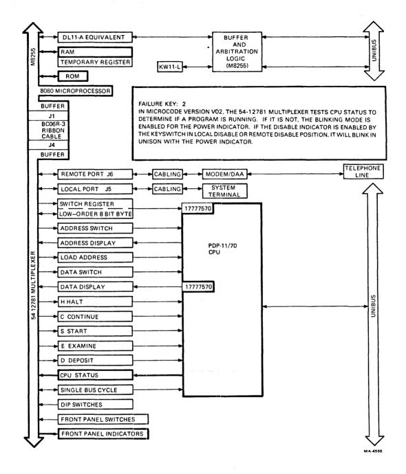
Figure 7-2 Failure Key 2
