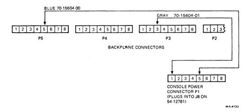
Figure 6-12 Power Jumper Installation
