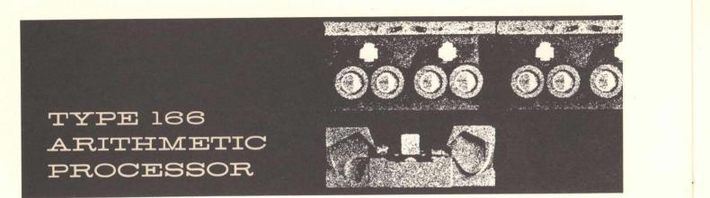
The Type 166 Arithmetic Processor is a general purpose processor capable of performing arithmetic, logical and input/output operations. It uses the first 16 locations in memory as accumulators, index registers, or ordinary memory locations. The results of each operation are transmitted automatically to one of these registers at the end of each instruction; thus the accumulator resides in memory.
