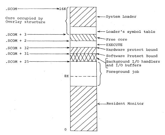
The System Loader loads EXECUTE's I/O handler (if not in core) in order to read the XCT file. The core limits of the overlay structure and the I/O requests in the .IODEV bit map are read from the XCT file. The user's I/O handlers and I/O buffers are then laoded above EXECUTE's handler, and the hardware protect bound is established above them. EXECUTE is loaded above the bound and Background free core is set up from the top of EXECUTE to the bottom of the overlay area.
