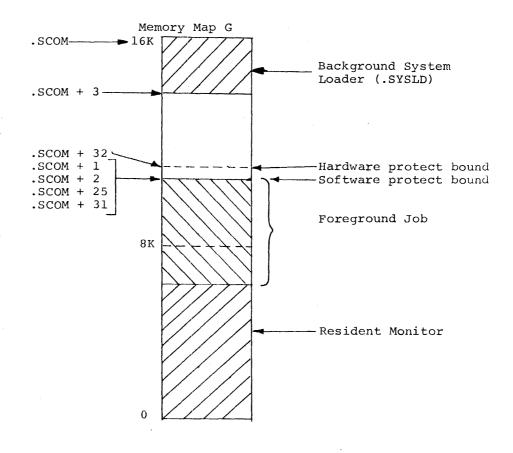
When a BACKGROUND keyboard command requests loading of a system or user program, the Non-resident Monitor brings in the System Loader, overlaying itself. Note that the BACKGROUND System Loader and the FOREGROUND Linking Loader are physically the same program.
