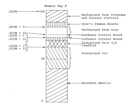
The .EXIT from the Linking Loader causes the user program I/O handlers to be block transferred to their running position, the memory protect bound to be set just above the I/O buffer space, and control given to the user program. if DDT was also loaded, it resides at the top of core, above the user programs. Its symbol table, built by the Loader, is block transferred by the Monitor to start at the software protect bound.
