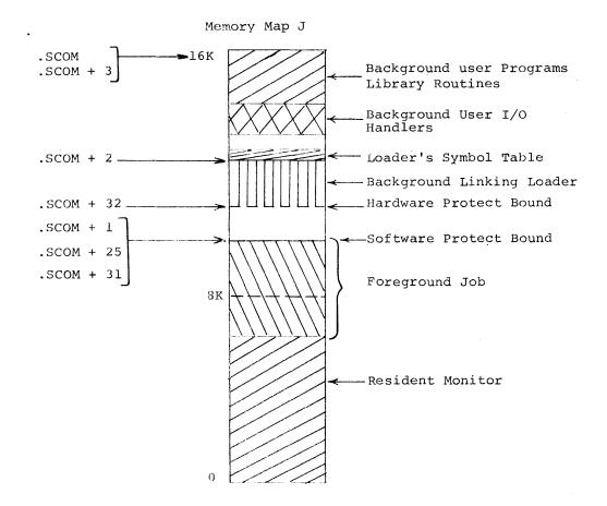
The BACKGROUND Linking Loader overlays the System Loader by loading user programs down from the top of core. User I/O handlers, presuming that they cannot fit in core between the FOREGROUND job and the bottom of the Loader, are loaded into upper core but relocated to run just above the FOREGROUND job so that they memory protect bound can be set above them. Common blocks and I/O buffers are not shown in this memory map.
