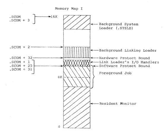
If the BACKGROUND program is a user program\*, the System Loader loads the Linking Loader I/O handlers up from the top of the FOREGROUND job and loads the Linking Loader such that the memory protect bound can be set just below it.
