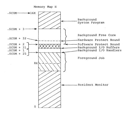
If the BACKGROUND request is for a system program, the System Loader loads the system program I/O handlers up from the top of the FOREGROUND job, allocates I/O buffer space, and loads the system program at the top of core (overlaying the System Loader). Control is returned to the Resident Monitor, which sets the memory protect bound above the buffer space and given control to the system program.
