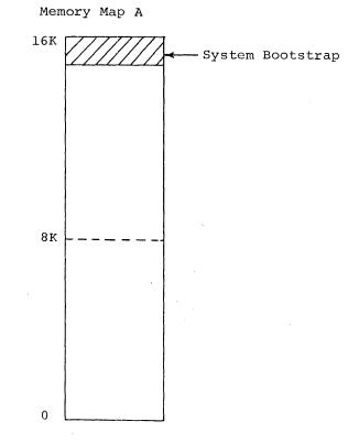
The System Bootstrap is loaded at the top of core via the paper tape reader in HRM format.
