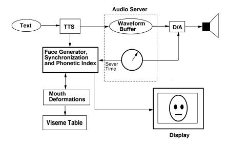
Figure 1: The synchronization model TTS = text-to-speech.
