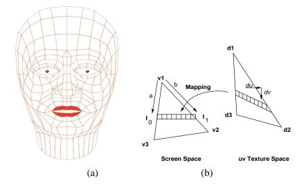
Figure 2: (a) Polygonal representation of the face. (b) Texture mapping.
