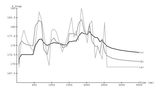
Figure 3: The mid top lip vertical displacement trajectories of the sample sentence. Trajectory (**a**) is the cosine activity peaking at each phonetic mouth shape. Trajectory (**b**) is the physical model with a small damping coefficient and a large spring constant, while trajectory (**c**) is the physical model with a larger damping coefficient and lower spring constant.
