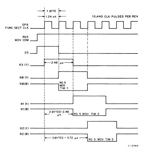
Figure 3-1 Move Timing Diagram
