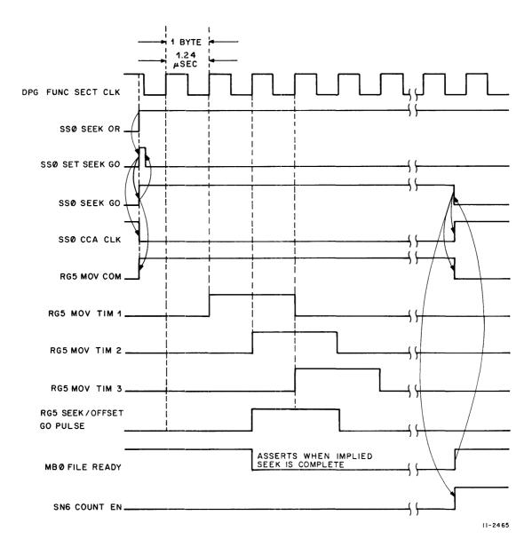
Figure 3-2 Implied Seek Timing Diagram
