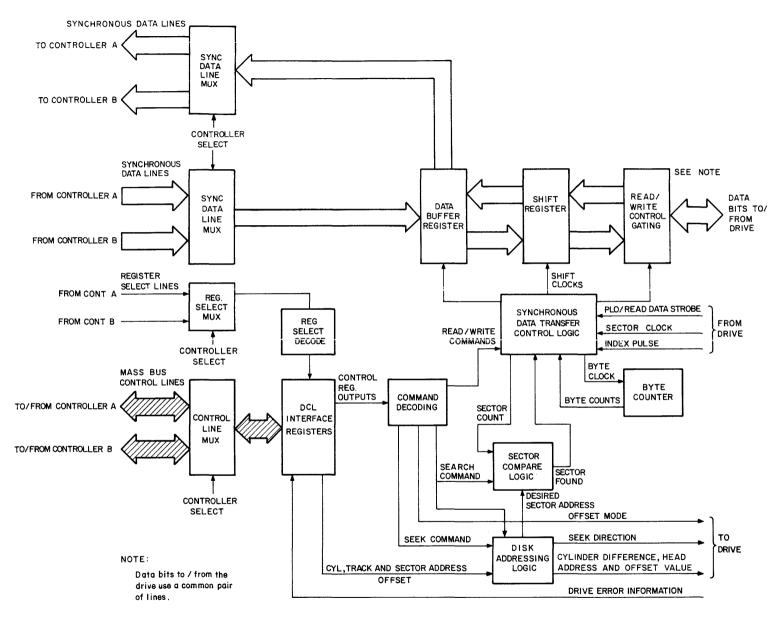
Figure 2-1 Device Control Logic, Simplified Block Diagram
