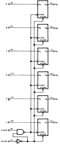
Pin (16) =  $V_{CC}$ , Pin (8) = GND
