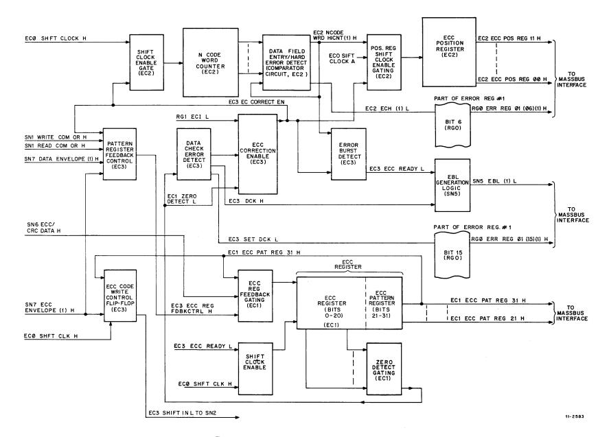
Figure 2-8 Error Correction Logic Block Diagram
