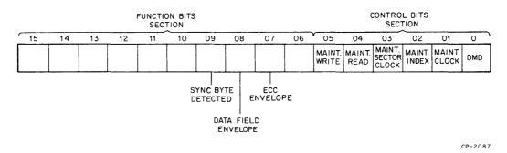
The Diagnostic Mode (DMD) bit must be set before the DCL can be placed in a diagnostic mode. With this bit set, the device handles the same command repertoire as it normally does.
