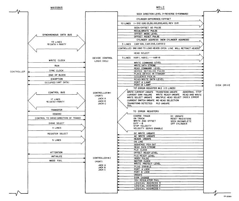
Figure 2-2 Massbus and MDLI (Drive) Interface Signals
