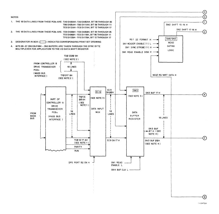
Figure 2-4 Synchronous Data Transfer Path Block Diagram (Sheet 1 of 2)
