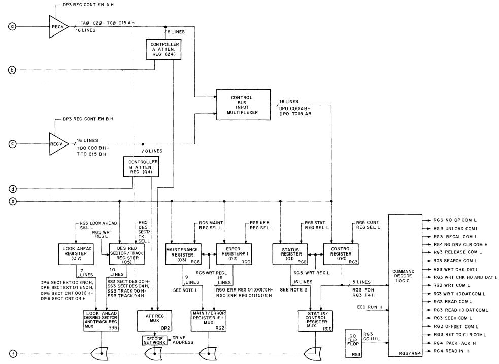
Figure 2-3 DCL Interface Registers and Massbus Control Signal Routing Block Diagram (Sheet 2 of 2)
