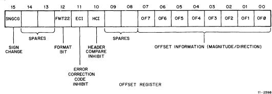
Bit 0-7 contain offset information which dictates how far (in microinches) from the centerline the read/write heads are to be positioned to implement the data recovery operation.
