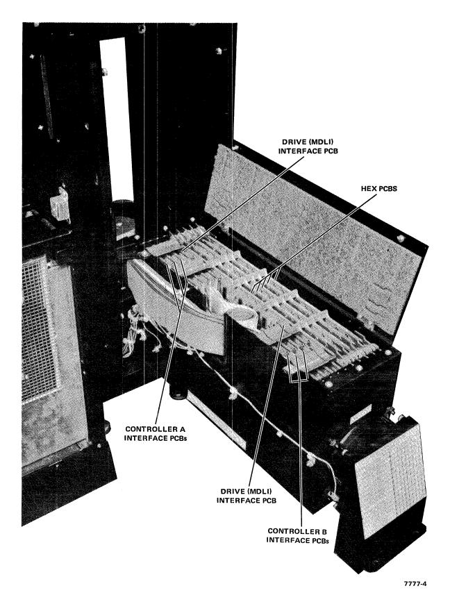
Figure 1-4 Card Nest and Cable Assembly PCB Layout
