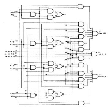
Pin (16) =  $V_{CC}$ , Pin (8) = GND
