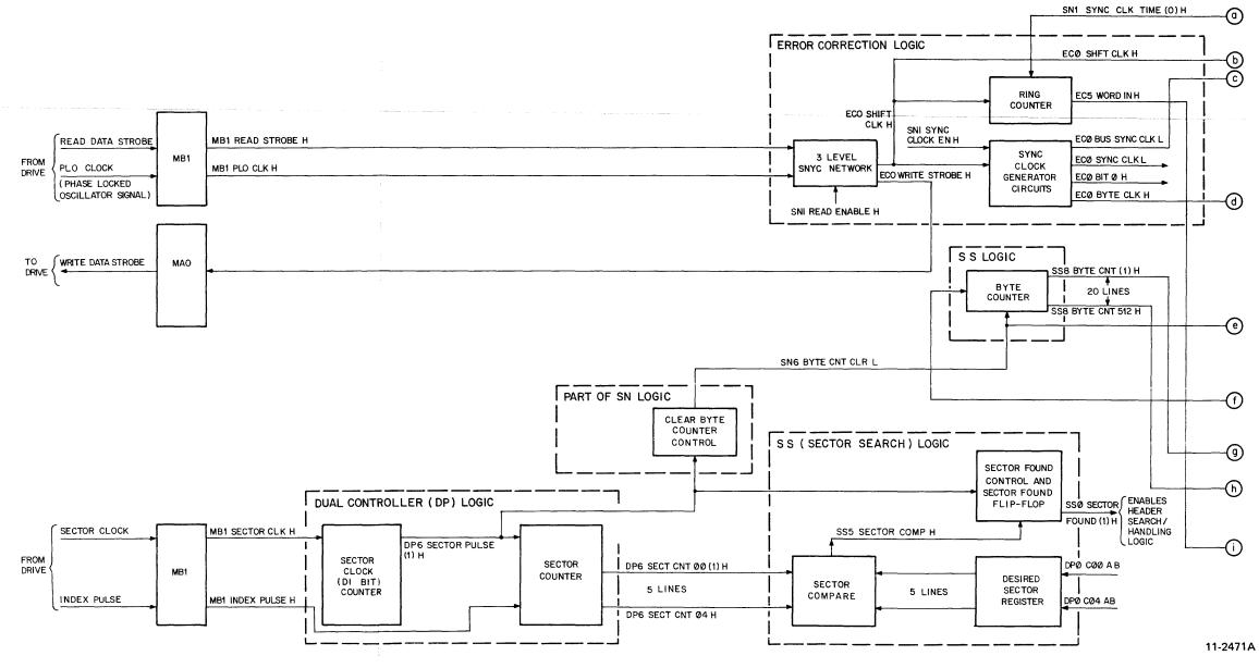
Figure 2-5 Basic Clock and Index Pulse Distribution Block Diagram (Sheet 1 of 2)
