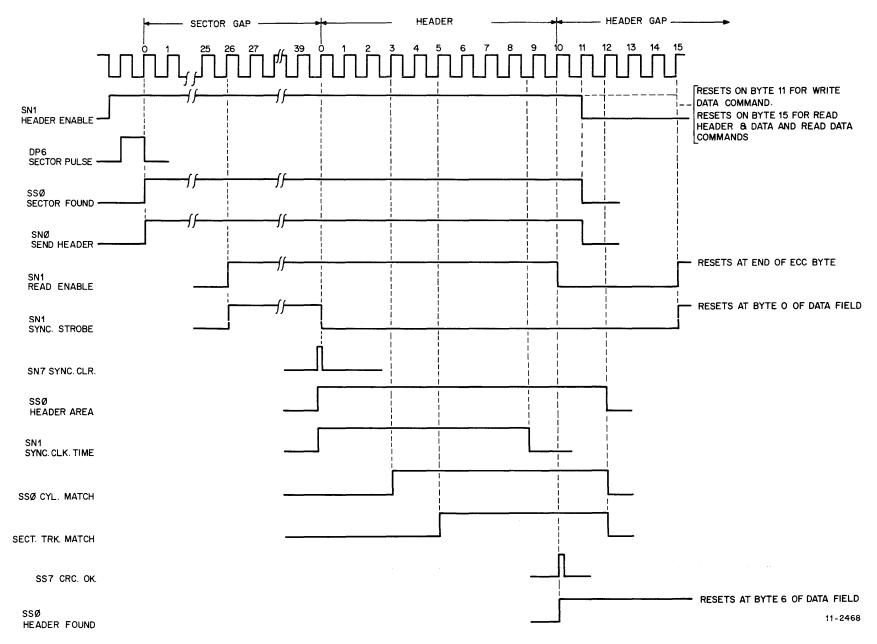
Figure 3-5 Header Compare Timing Diagram
