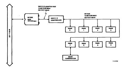
Figure 1 RKV11-D/RK05 System Configuration
