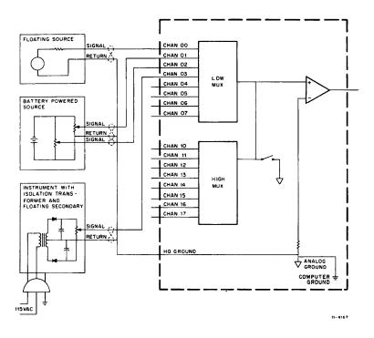
Figure 8 Floating ADV11-A Input Signals
