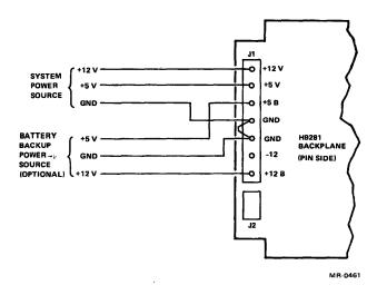
Figure 3 H9281 Power Connections
