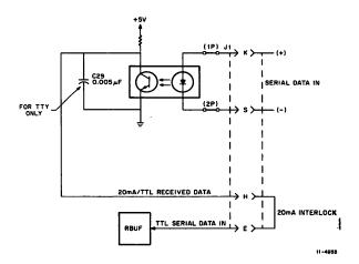
Figure 12 Passive Receive 20 mA Current Loop
