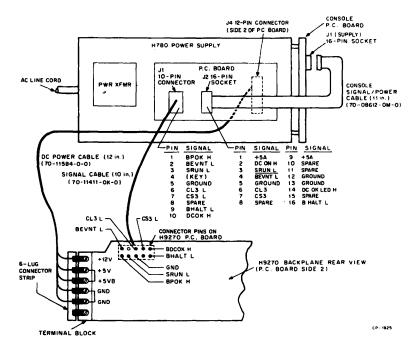
Figure 19 H780 to H9270 Backplane Connections
