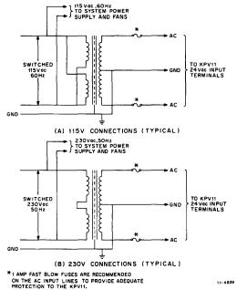
Figure 10 Power Line Monitor Transformer Installation
