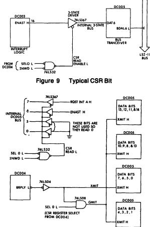
WHEN THE CSR IS READ (SEL 0 L = 0) THE SIGNAL GMIT WILL BE 0 CAUSING THE UNUSED DC005 BITS TO BE READ AS ZEROS. (HIGH ON BDAL LINES) FOR ANY OTHER REGISTER GMIT = XMIT.
