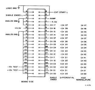
Figure 11 ADV11-A 40-Pin Connector Pin Assignments
