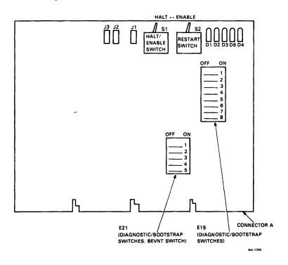
Figure 4 BDV11 Switches and Indicators
