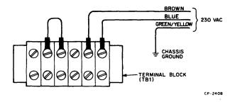
Figure 14 H780-D, -J, and -L (230 Vac) AC Terminal Block Wiring Configuration
