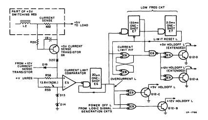
Figure 7 Overload and Short-Circuit Protection Circuits
