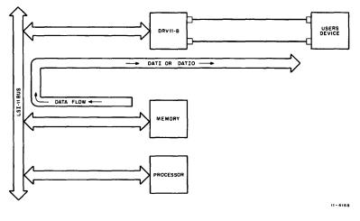
Figure 3 DMA DATIO/DATI Data Flow Diagram
