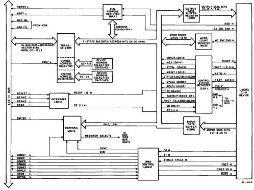
Figure 1 DRV11-B Logic Block Diagram
