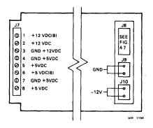
Figure 2 H9273-A Power Connections
