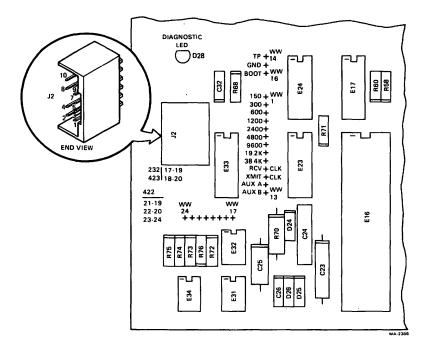
Figure 13 Interface Selection Jumper Pin Locations
