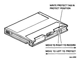
Figure 6 Write Protect Tab
