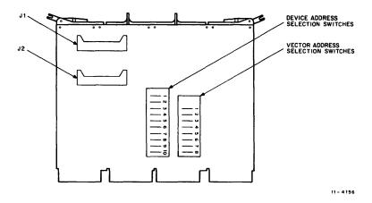
Figure 8 DRV11-B Connector and Switch Locations
