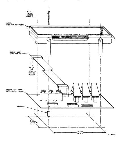
Figure 11 Console Panel Installation
