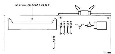
Figure 13 EIA Jumper Configuration
