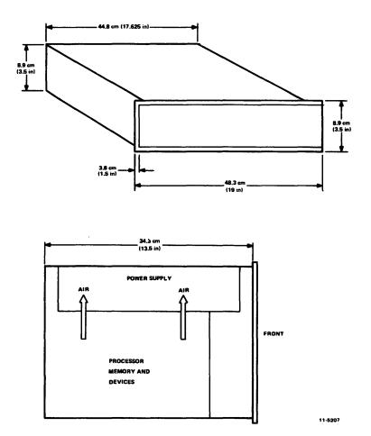
Figure 2 BA11-M Assembly Unit
