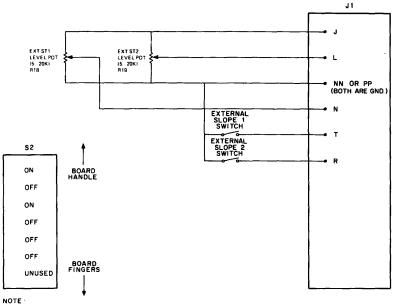
For proper operation of external level controls, both R18 and R19 on KWVII-A board must be set to approximate mid-point of rotation, and the S2 switches must be set as shown.
