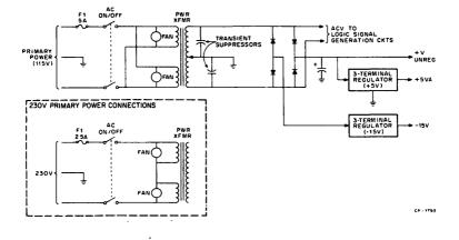
Figure 5 Unregulated Voltage and Local DC Power Circuits
