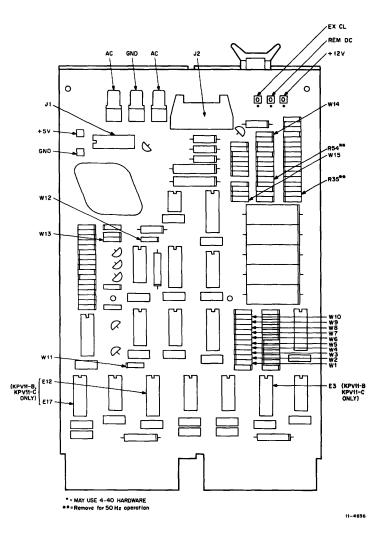
Figure 7 Jumper, Connector, Resistor, and Pad Locations
