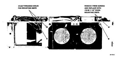
Figure 17 Left Side of H780 Showing H9270 Mounting Holes
