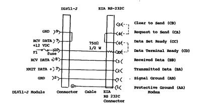
Figure 7 BC21B-05 Modem Cable
