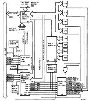
Figure 1 Bus Interface, I/O Control, and Interrupt Logic
