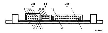
Figure 4 Connector Pin Number Location Diagram
