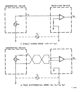
Figure 9 Single-Ended vs. True Differential Input Modes
