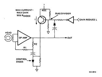
Figure 19 Read Amplifier and Automatic Gain Control
