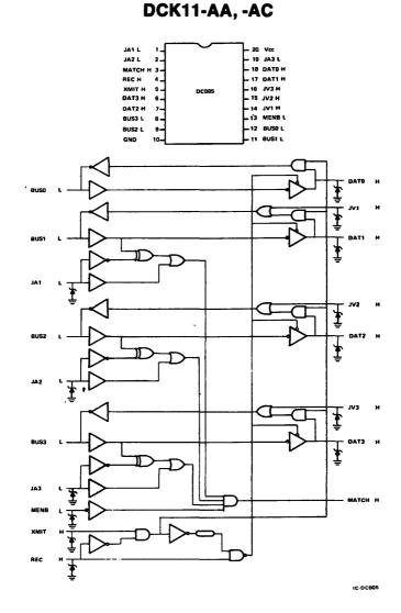
Figure 4 DC005 Simplified Logic Diagram
