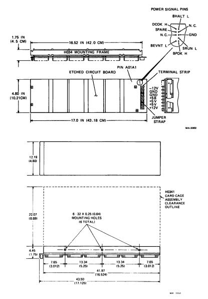
Figure 3 DDV11-B Power Wiring and Dimensions
