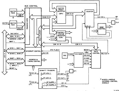
Figure 1 KWV11-A Real-Time Clock Block Diagram
