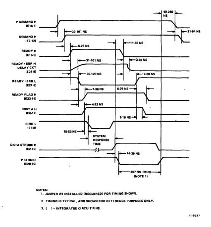
Figure 3 LA180 Internal Timing
