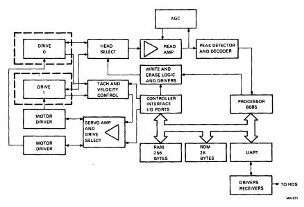
Figure 3 TU58 Block Diagram
