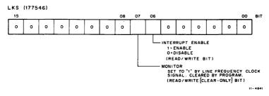
Figure 15 Line-Time Clock Status Register (LKS)
