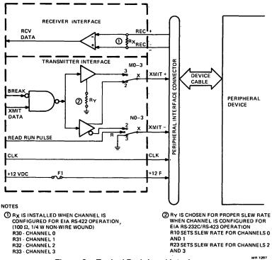
Figure 2 Typical Peripheral Interface
