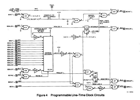
console LTC ON/OFF switch enable/disable, and manual/-programmable operation. Additional jumpers (W1-W10) select the device address for the LKS register. Jumpers are factory-configured as shown in Figure 8.
