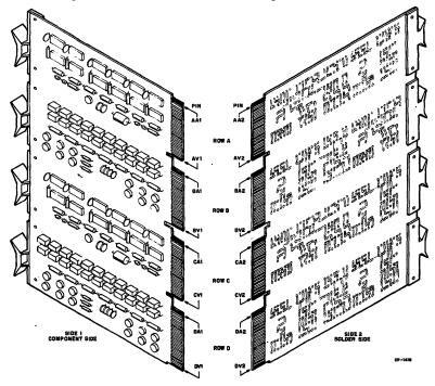
Figure 2 Quad Module Contact Finger Identification
