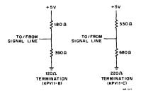
Figure 5 KPV11-B and KPV11-C Bus Terminations
