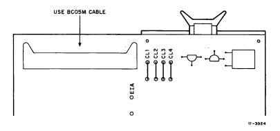
Figure 8 20 mA Active Current Loop Jumper Configuration
