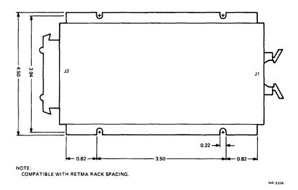
Figure 5 DLV11-KA Mounting Dimensions
