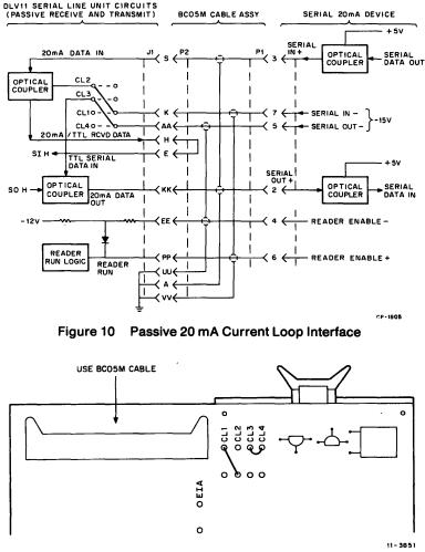
Figure 11 20 mA Passive Current Loop Jumper Configuration
