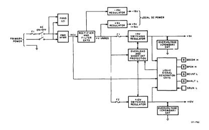
Figure 4 H780 Power Supply Block Diagram
