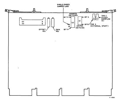
Figure 2 ADV11-A Connectors and Switches
