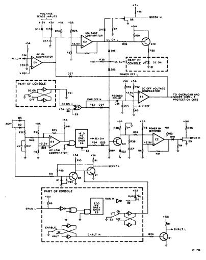
Figure 9 Logic Signal Generation Circuits
