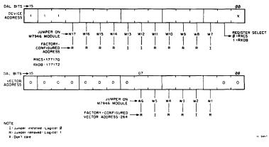
Figure 2 Device Register Address and Interrupt Vector
