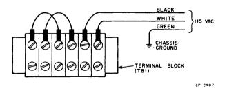
Figure 13 H780-C, -H, and -K (115 Vac) AC Terminal Block Wiring Configuration
