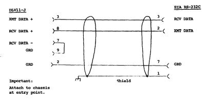
Figure 8 BC20N-05 "Null Modem" Cable
