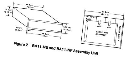
The ac input box, power supply, and H9273 logic assembly are attached to the logic box base. The power supply assembly is hinged to the base and can be swung open to expose the internal components; with little effort, the entire assembly can be removed from the base and replaced. LSI-11 bus modules are inserted in the backplane from the rear of the box through an access door that is equipped with strain reliefs for LSI-11 bus and communications cables.
