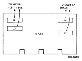
Figure 6 M7268 Cable Connections
