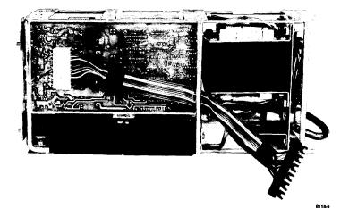
Figure 22 H780 DC Output Connector (J4) with Mating DC Output Cable (70-11584-0-0)
