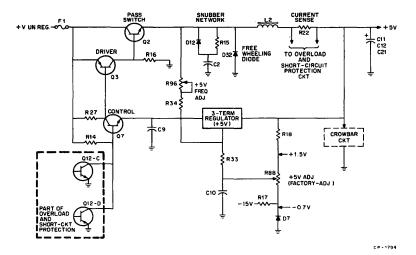
Figure 6 Basic Regulator Circuit
