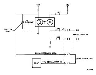
Figure 11 Active Receive 20 mA Current Loop
