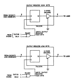
Figure 6 Example of Output Register
