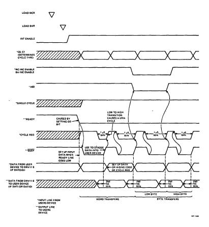
Figure 5 DRV11-B Timing: Single Cycle, Asynchronous, Program-Initiated
