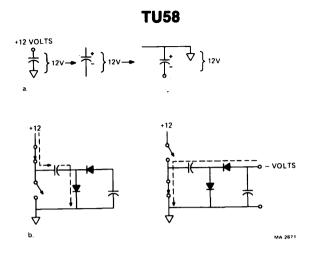
Figure 20 Simplified Charge Pump
