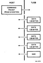
Figure 8 Read Command Packet Exchange
