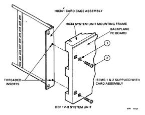
Figure 4 H0341 Card Assembly Installation
