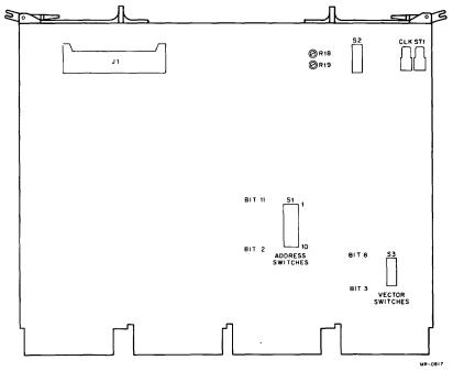
Figure 2 KWV11-A Connectors, Switches, and Controls
