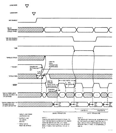
Figure 6 DRV11-B Timing: Burst Mode, User-Initiated
