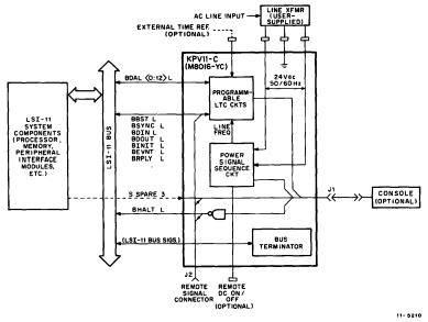
Figure 1 KPV11 Functional Block Diagram
