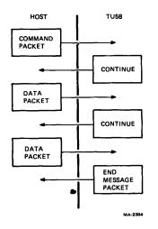
Figure 2 An Exchange in Radial Serial Protocol
