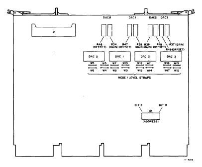
Figure 2 AAV11-A Connectors, Switches, and Jumpers
