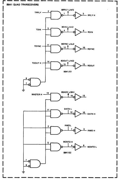
Figure 5 Typical Application (Miscellaneous Logic) (Sheet 3 of 3)
