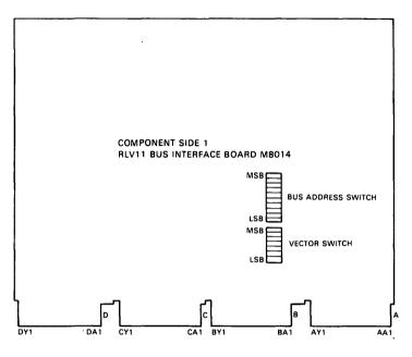
Figure 2 RLV11 Bus Interface Module (M8014)
