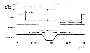
Figure 11 DC ON/OFF Circuit Timing
