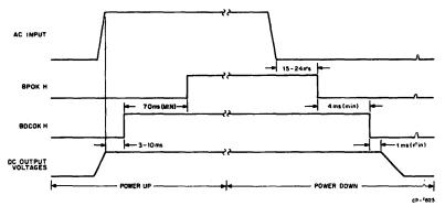
Figure 10 Power-Up/Power-Down Sequence
