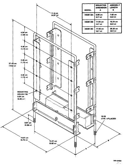
Figure 2 H9281-BA, BB, BC Mounting Dimensions
