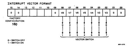
Figure 4 RLV11 Interrupt Vector Format
