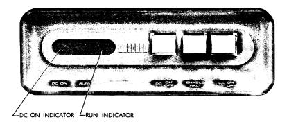
Figure 12 Console Panel Controls and Indicators (P/N 54-11808 and 70-11656 shown)
