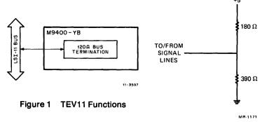
Figure 2 Typical 120-Ohm Bus Termination
