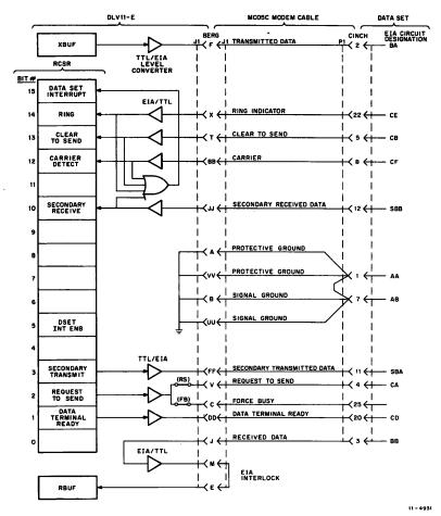
Figure 9 DLV11-E Peripheral Interface Signal Flow
