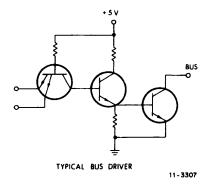
Figure 2 Typical Bus Driver Circuit
