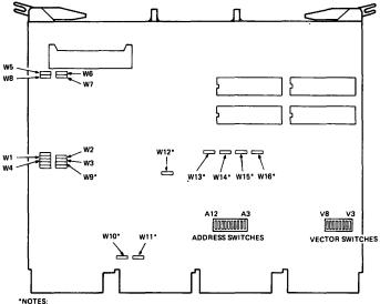
JUMPERS W9, W12, W13, W14, W15, AND W16 ARE REMOVED ONLY FOR MANUFAC-TURING TESTS. THEY SHOULD NOT BE REMOVED IN THE FIELD.
