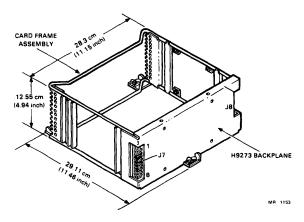
Figure 1 H9273-A Backplane Logic Assembly
