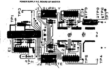
J2 (REMOTE) CONNECTED TO J2 (REMOTE) ON SLAVE SUPPLY INDICATOR P.C. BOARD
