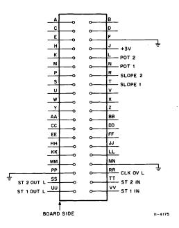
Figure 8 J1 40-Pin Connector Pin Assignments
