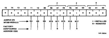
Figure 4 M7269 Interrupt Vector Format
