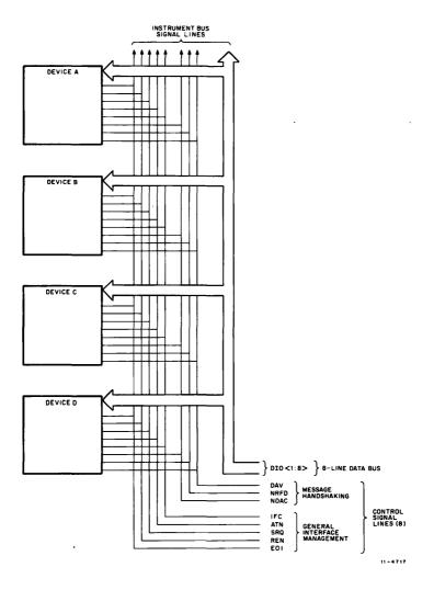
Figure 5 Instrument Bus Signal Lines
