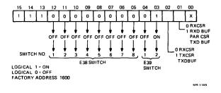
Figure 3 Device Address Selection
