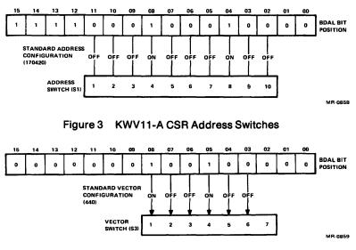
Figure 4 KWV11-A Vector Address Switches
