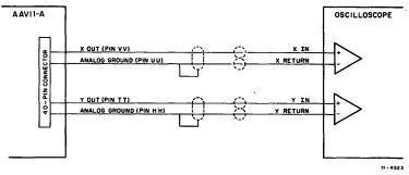
Figure 5 J1 Connector Pin Assignments
