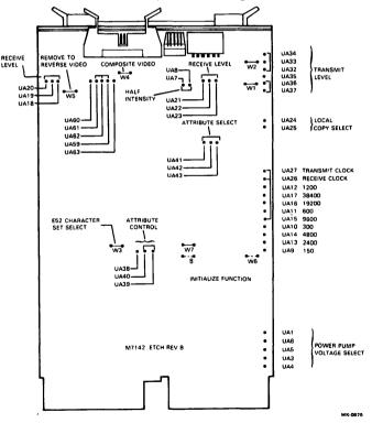
Figure 6 Jumper and Wire Wrap Post Locations
