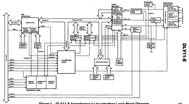
Figure 1 DLV11-E Asynchronous Line Interface Logic Block Diagram
