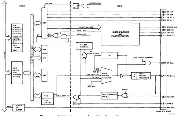
Figure 1 RLV11 Controller Simplified Block Diagram
