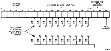
Figure 3 DRV11-P Device Address Select Format
