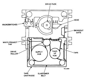
Figure 5 Tape Cartridge Partially Inserted Into Drive
