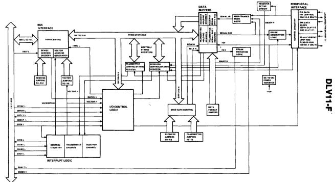
Figure 1 DLV11-F Asynchronous Line Interface Logic Block Diagram
