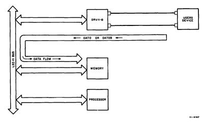
Figure 2 DMA DATO/DATOB Data Flow Diagram
