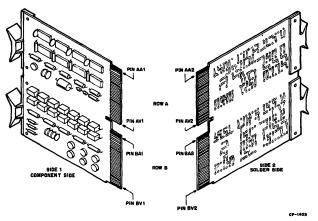
Figure 1 - Dual Module Contact Finger Identification
