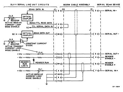
Figure 9 Active 20 mA Current Loop Interface
