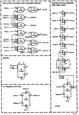
Figure 5 Typical Application (Miscellaneous Logic) (Sheet 1 of 3)
