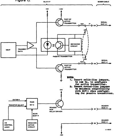
Figure 10 20 mA Transmitter and Reader Run Circuits
