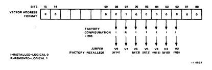
Figure 6 LPV11 Interrupt Vector Format and Jumpers
