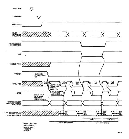
Figure 4 DRV11-B Timing: Single Cycle, Asynchronous, User-Initiated
