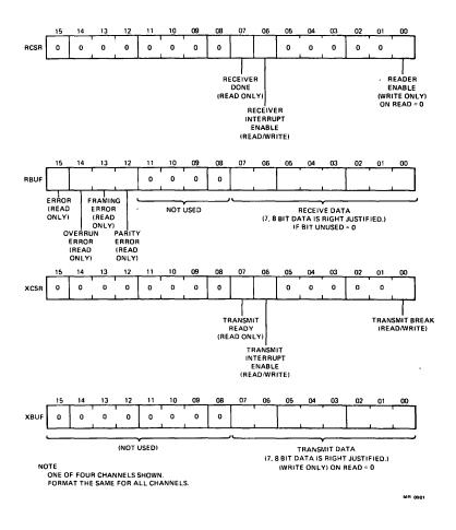
Figure 5 DLV11-J Device Register Formats
