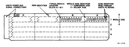
Figure 3 LSI-11 Backplane Module Pin Identification
