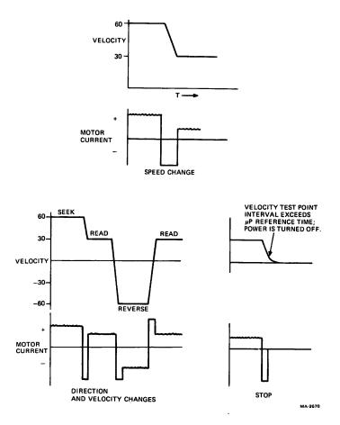
Figure 17 Velocity Change Waveforms
