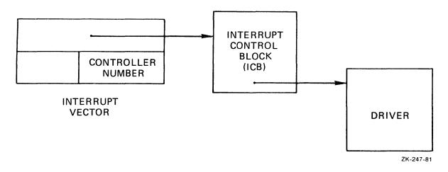
Figure 1-2: Interrupt Dispatching for a Driver
