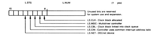
Figure 4-17: Controller Table Status Byte
