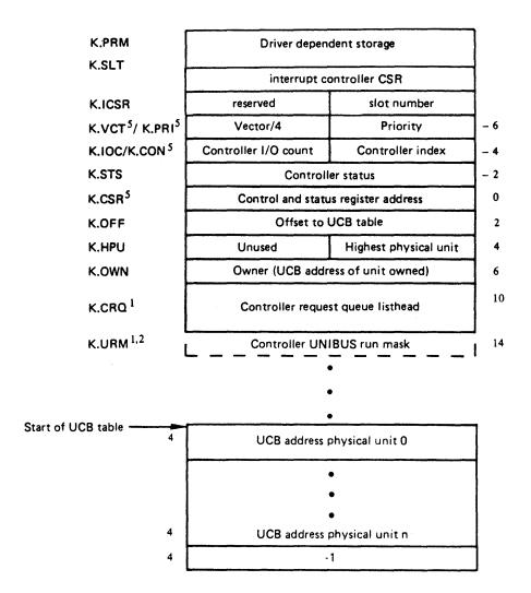
Figure 4-13: Controller Request Block
