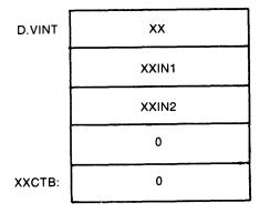
Figure 4-19: Sample Interrupt Address Block in the DDT
