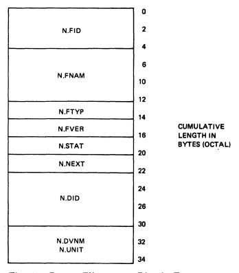
Figure D-1: Filename Block Format
