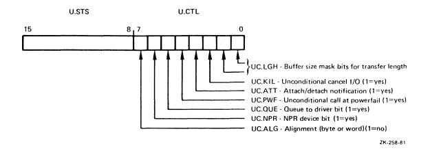
Figure 4-7: Unit Control Byte
