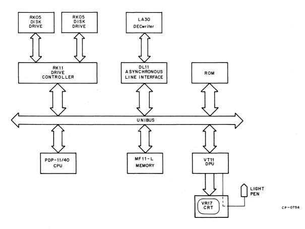
Figure 1 Relationship of GT44 Components to the Unibus
