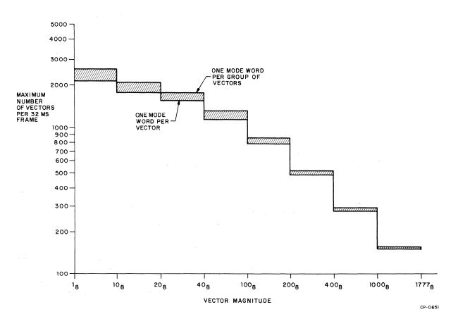
Figure 8 Non-Flicker Display as Determined by Vector Quantity and Magnitude
