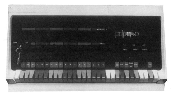
Figure 2 PDP-11/40 Programmer's Console
