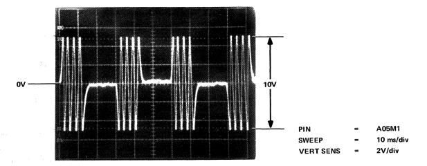
a. Correct Waveform (Symmetrical Signal)
