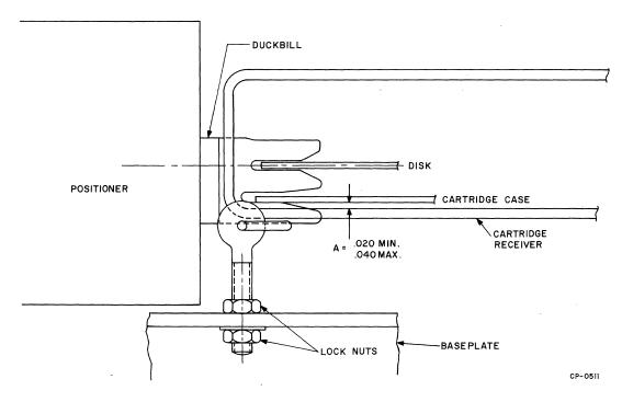
Figure 5-21 Cartridge to Receiver Clearance
