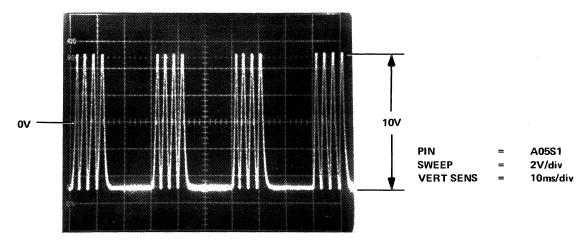
Figure 5-12 Cosine Amplitude/Offset Waveform
