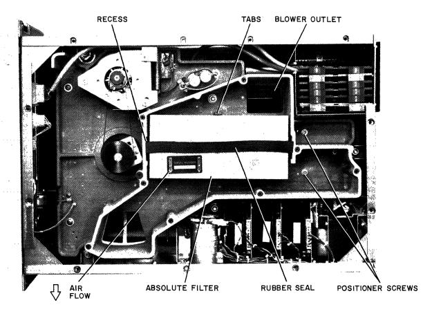
Figure 5-2 Absolute Filter Removal
