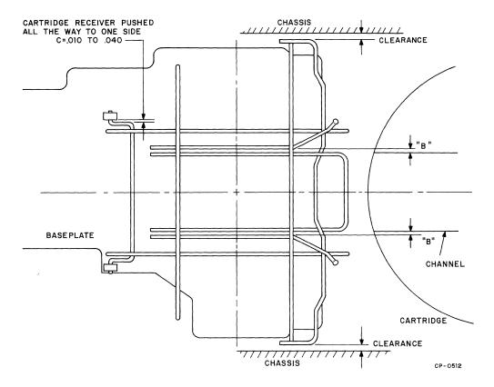
Figure 5-22 Cartridge Receiver Clearances
