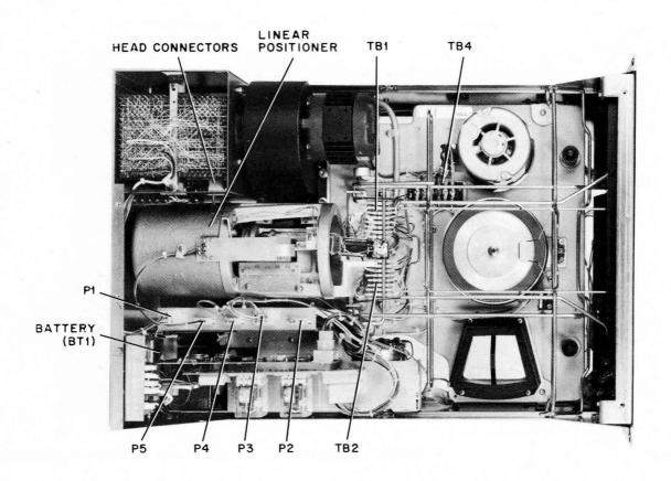
Figure 5-3 Top View with Cover Removed
