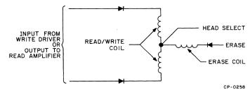
4.1.5 Recording Technique Figure 4-7 Simplified Read/Write Head Circuit
