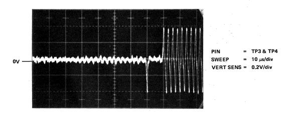
Figure 5-18 Index/Sector Waveform
