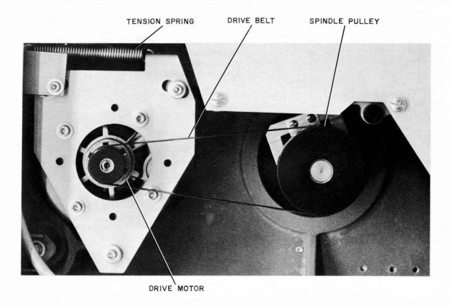
Figure 1-3 Spindle and Drive System
