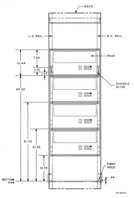
Figure 2-2 Chassis Slide Mounting
