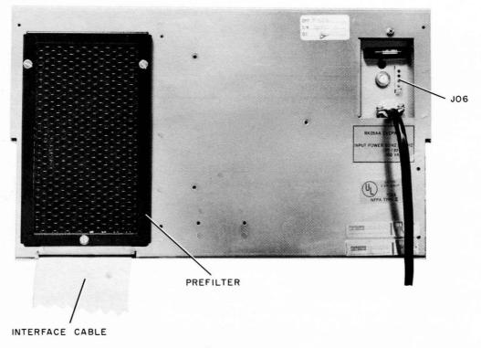
Figure 2-3 RK11C or RK11D Interface Cable Installation
