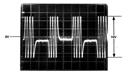
b. Incorrect Waveform (Signal not Symmetrical about Ground)
