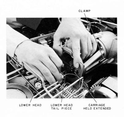
b. Lower Head Removal and Installation
