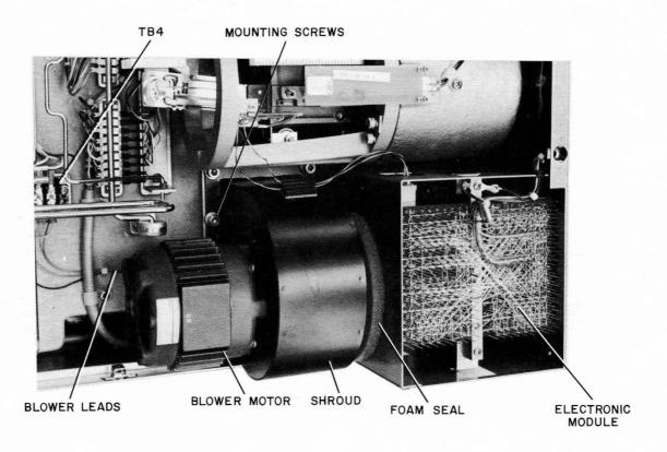
Figure 5-9 Blower Motor Removal
