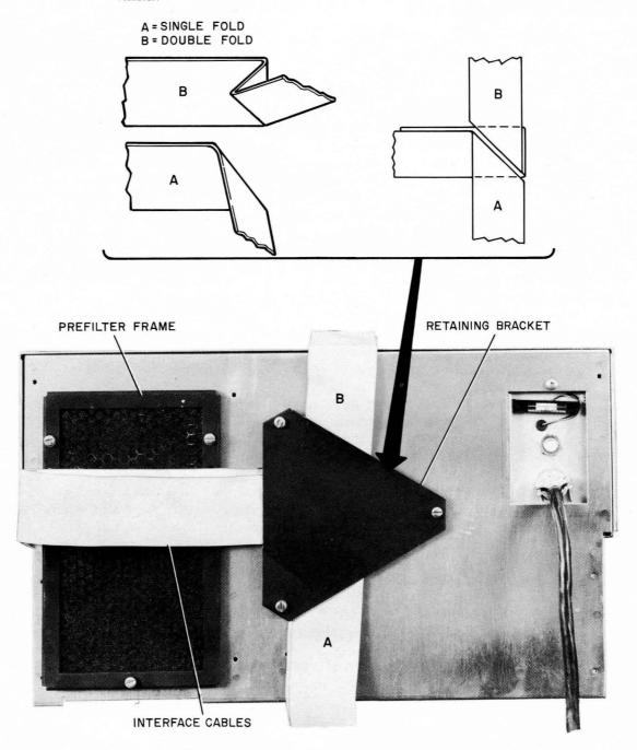
Figure 2-4 RK8/E Interface Cable Installation (Preferred Method)
