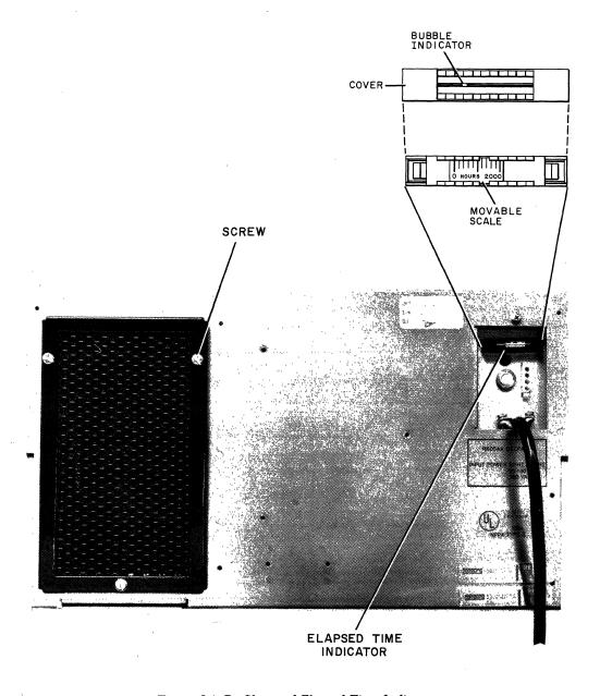
Figure 5-1 Prefilter and Elapsed Time Indicator
