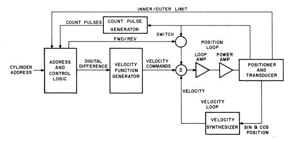
Figure 4-12 Servo System Block Diagram
