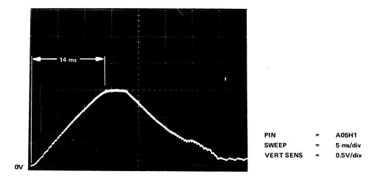
Figure 5-14 Acceleration Waveform
