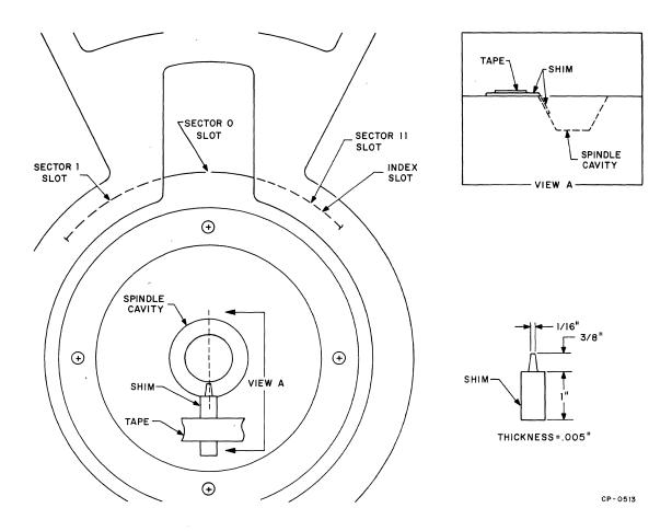
Figure 5-10 CE Test Cartridge Shim Installation
