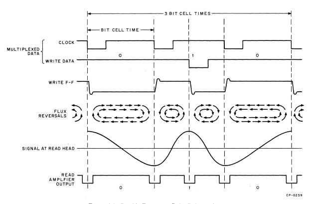
Figure 4-9 Double Frequency Pulse Relationship
