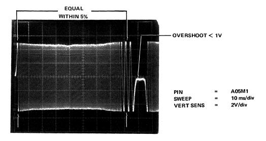
Figure 5-16 Full Stroke Position Waveform
