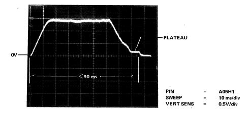
Figure 5-15 Full Stroke Waveform
