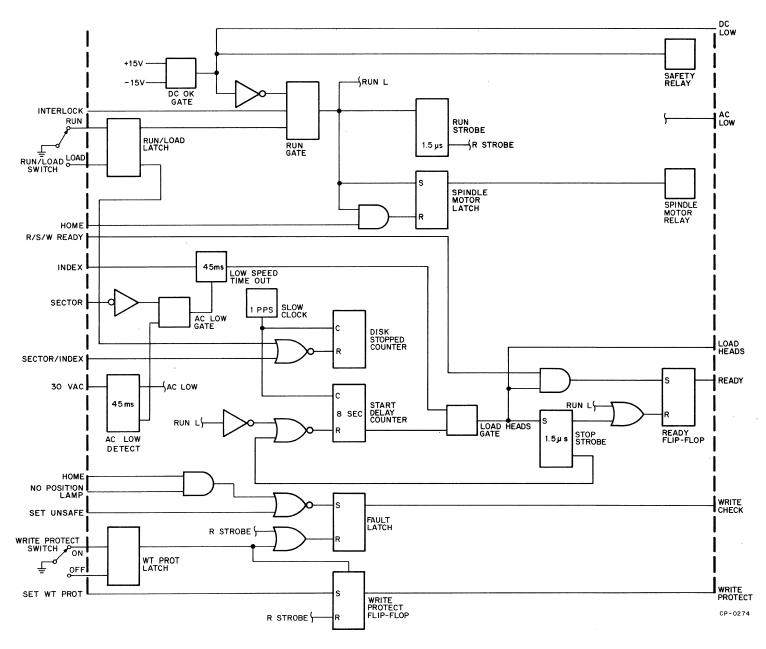
Figure 4-10 Control and Interlock Block Diagram
