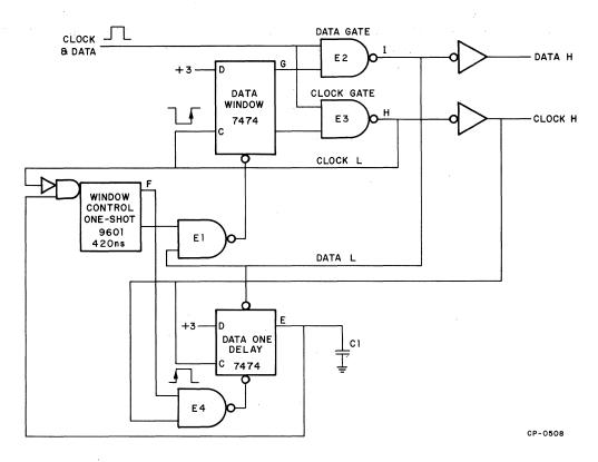
Figure 4-16 Simplified Data Separator Circuit
