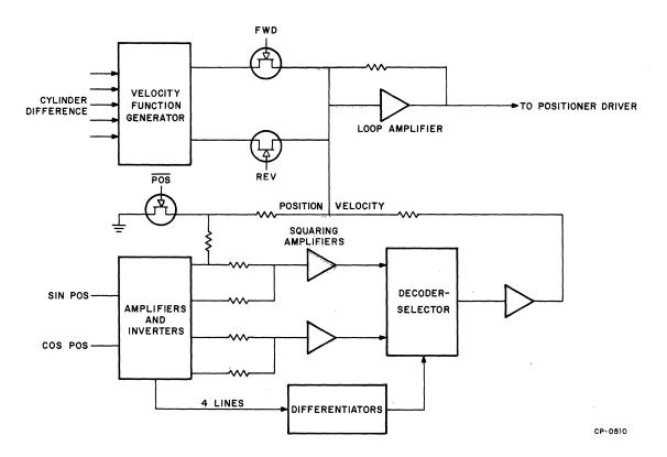
Figure 4-14 Simplified Positioner Servo Logic
