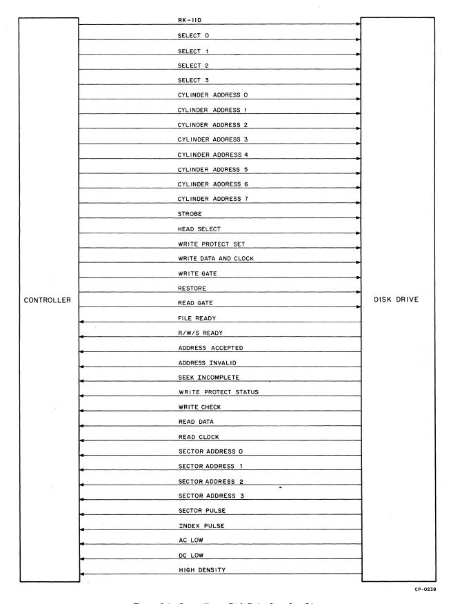
Figure 3-1 Controller to Disk Drive Interface Lines
