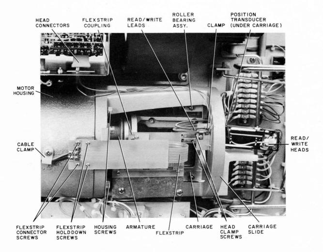
Figure 5-4 Carriage Removal
