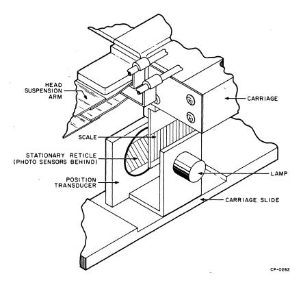
Figure 4-13 Linear Positioner Transducer
