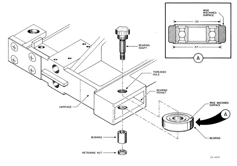
Figure 5-5 Carriage Bearing Assembly Removal
