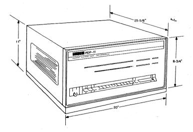
Figure 6.3 Table Top PDP-11 Dimensions
