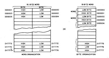
PDP-11 memories are normally provided in 4096-word read and write modules. However, there are also 8192-word interleaved memory modules. The various PDP-11 memories, their characteristics and speeds are listed below.
