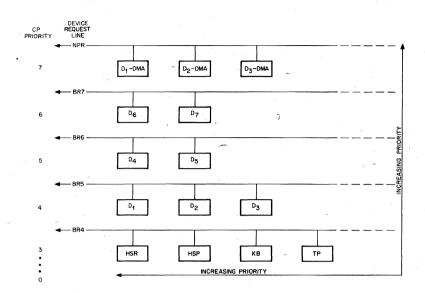
See Table 1-1, page 2, for a summary of the API structures of the various PDP-11's. Bus requests from external devices can be made on one of five request lines. Highest priority is assigned to non-processor request (NPR). These are direct memory access type transfers, and are honored by the procesor between bus cycles of an instruction execution.
