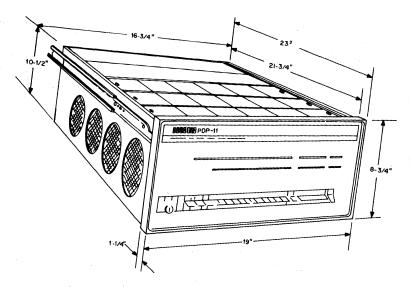
Figure 6.4 Rack-Mountable PDP-11 Dimensions
