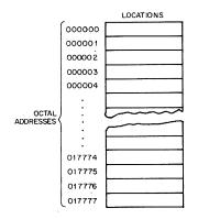
Because PDP-11 memories are designed to accommodate both 16-bit words and 8-bit bytes, the total number of addresses does not correspond to the number of words. A 4096-word memory can contain 8,192 bytes and consists of 017777 octal locations. Words always start at even-numbered locations.
