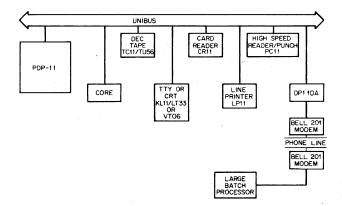
Figure 2-3 Remote Terminal Controller
