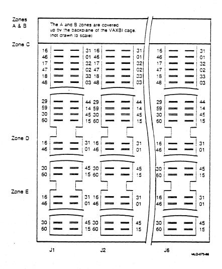
Figure 13-10: Reference Designation for Connector Pins
