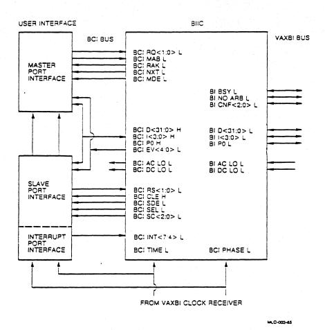
Figure 14-1: Block Diagram of a VAXBI Node
