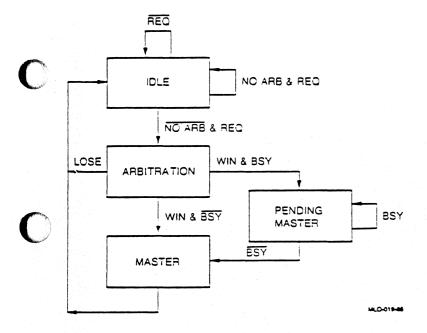
Figure 4-4: Arbitration State Diagram
