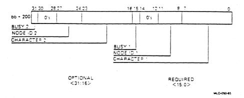
The Receive Console Data Register (RXCD), which is implemented by VAXBI nodes that have a console on the VAXBI, is used to receive data from other consoles. Nodes that do not implement a VAXBI console must respond to reads to the RXCD location with either a NO ACK response or return a longword of data in which the RXCD Busy 1 bit is set. In the latter case, the Busy 1 bit must be set before the Broke bit is cleared at the completion of self-test.
