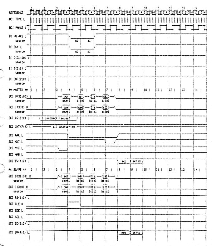
Figure 21-3: Loopback Longword Read-Type with a STALL
