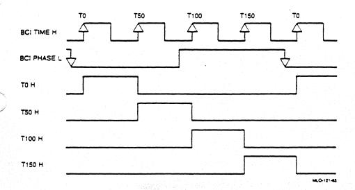
Figure AN6-4: Even Phase Clock Generator Logic
