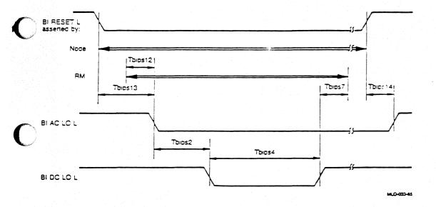
Figure 6-3: "Extended" System Reset Timing Diagram
