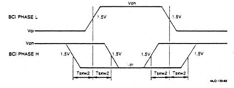
Figure AN6-3: Skew Between True and Complement Outputs of TIME and PHASE
