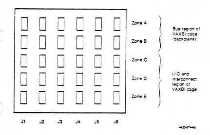
Figure 13-9: Reference Designation for Connector Zones
