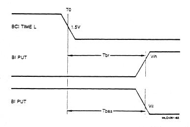
Figure 20-4: VAXBI Driver Output Waveforms
