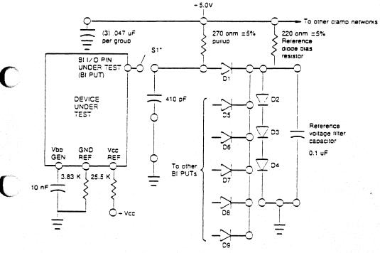
\*Switch S1 is closed for AC tests and open for DC tests.
