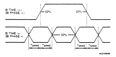
Figure 12-3: Differential Clock Skew
