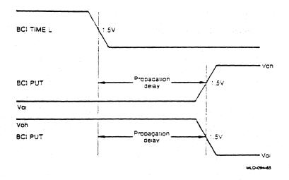
Figure 20-7: BCI Transceiver Propagation Delay Waveforms
