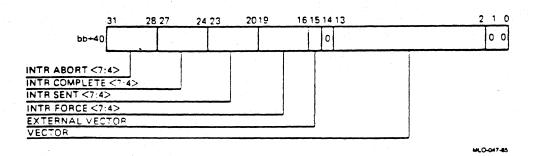
The User Interface Interrupt Control Register controls the operation of interrupts initiated by the user interface. In the following discussion, the phrase "interrupt request" refers to interrupts initiated either by the assertion of any of the BCI INT<7:4> L lines or by the setting of any of the force bits in this register.
