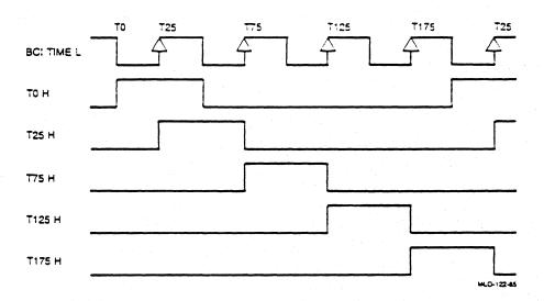
Figure AN6-5: Odd Phase Clock Generator Logic
