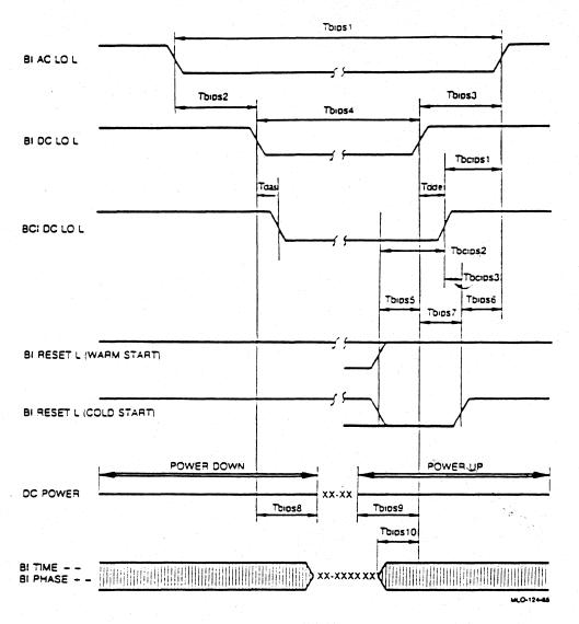
Figure AN7-1: System Reset Sequence
