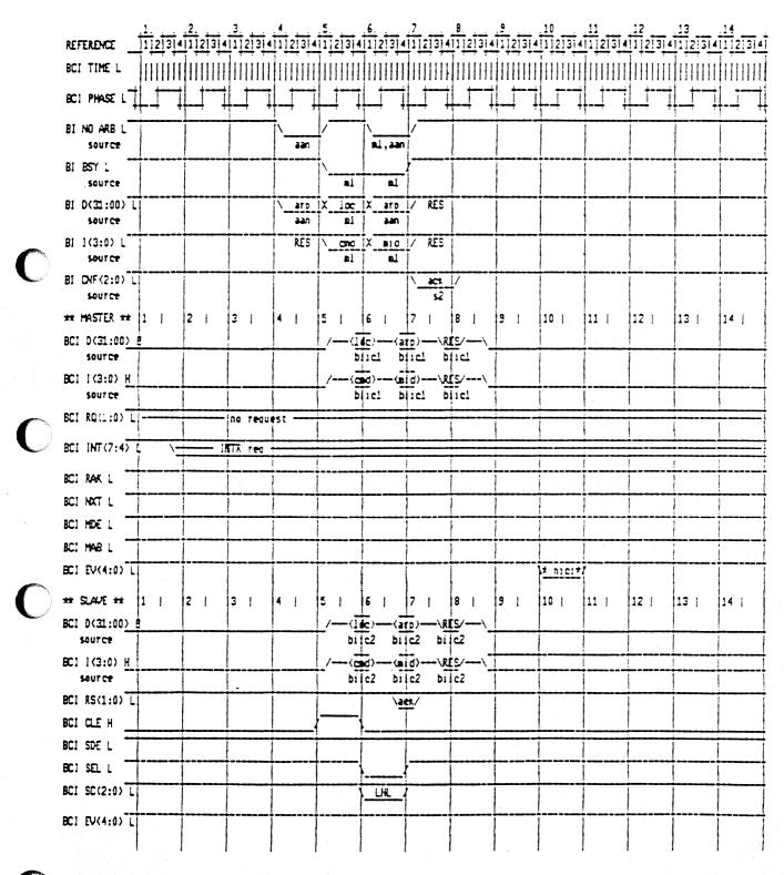
Figure 21-15: Master Port Interprocessor Interrupt
