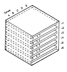
Legena: c cam actuator for ZIF s self-test LED o other LED(s) Notes: -Modules are horizontal -Backbiane is vertical, and in back of the modules Front entry for modules -Air flow is either: -eft to right, or -ngnt to left -Remote cam actuator -Components on top side of modules -VAXBI Comer at left rear of modules
