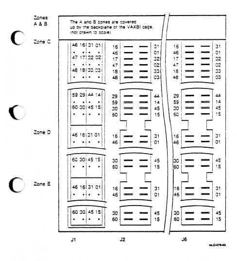
Figure 13-11: Reference Designation for Header Pins
