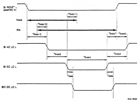
Figure AN7-3: System Reset Timing Diagram
