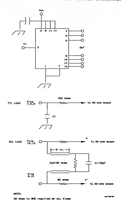
Figure 22-4: AC Test Fixture
