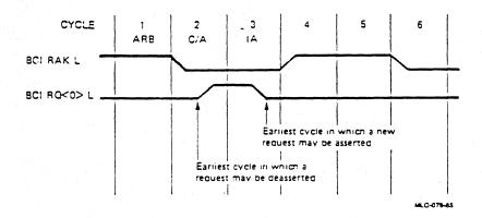
Figure 15-2: Pipeline-Request Signal Timing
