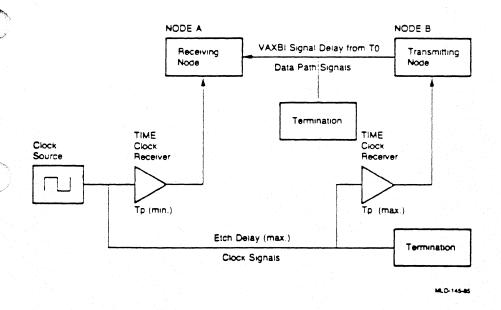
Figure 12-4: Worst-Case Setup Time Configuration
