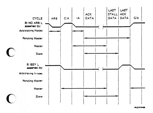
Figure 4-2: Transaction Showing BI NO ARB L and BI BSY L
