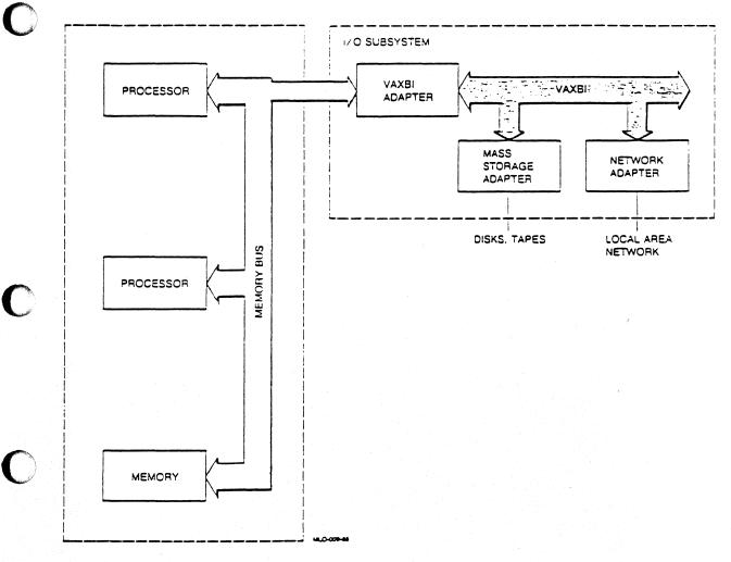
Figure 1-9: Multiprocessor High-End System Configuration
