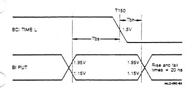
Figure 20-5: VAXBI Receiver Setup and Hold Time Waveforms
