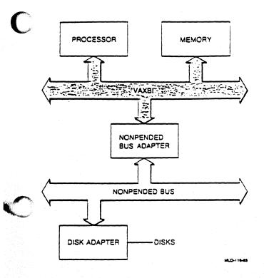
Figure AN5-2: Configuration with a Nonpended Bus Adapter
