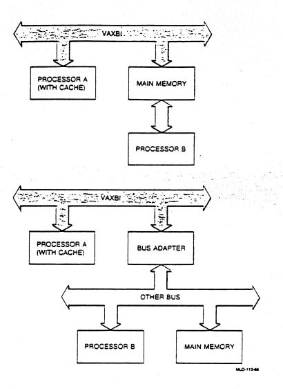
Figure AN2-2: Configurations with Nodes That Do Local Writes
