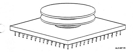
Figure 19-1: Packaged BIIC with Heat Sink
