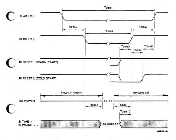
Figure 6-1: System Reset Sequence
