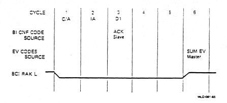
Figure 15-5: Summary EV Code Timing for Successful STOP, INTR, IPINTR, and INVAL Transactions
