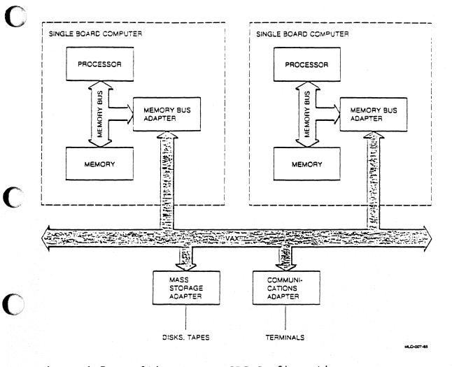
Figure 1-7: Multiprocessor SBC Configuration
