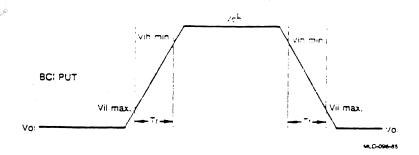
Figure 20-9: BCI Driver Rise and Fall Time Waveforms
