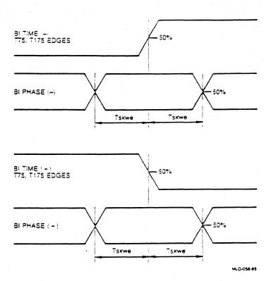
Figure 12-2: Edge-to-Edge Skew Between TIME and PHASE
