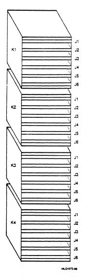
Figure 13-8: Reference Designation for Horizontal Module Mounting
