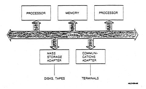
Figure 1-6: Multiprocessor Configuration
