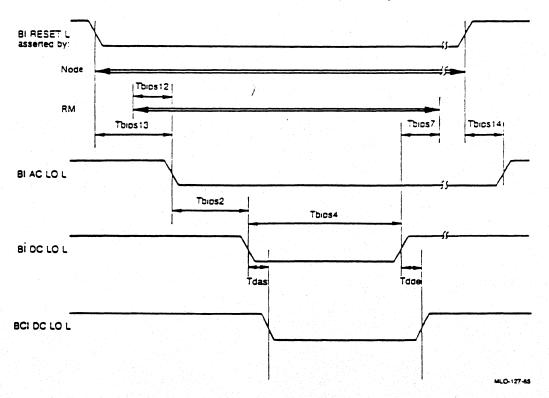
Figure AN7-4: "Extended" System Reset Timing Diagram
