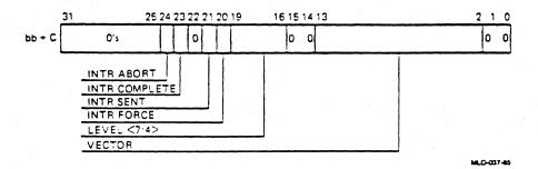
The Error Interrupt Control Register controls the operation of interrupts initiated by a BIIC-detected bus error (which sets a bit in the Bus Error Register) or by the setting of a force bit in this register. In the descriptions that follow, an error interrupt request can be initiated either by the setting of a force bit or by the setting of a Bus Error Register bit (assuming the appropriate error interrupt enables are set in the VAXBI Control and Status Register).
