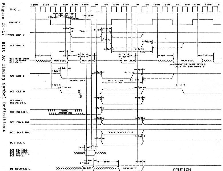
Note 1: This extended BCI data window is only usable in designs in which BCI MDE L never asserts (i.e., slave port only designs such as memory), and even in these designs it only applies to data cycles (i.e., command/address cycles still have the narrow window).
