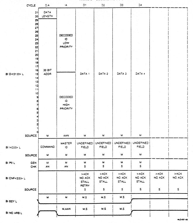
Figure 5-2: WRITE and WCI Transactions (octaword length shown)
