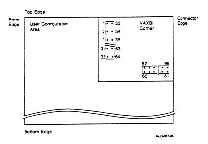
Figure 13-2: VAXBI Corner Signal Locations (component side view)
