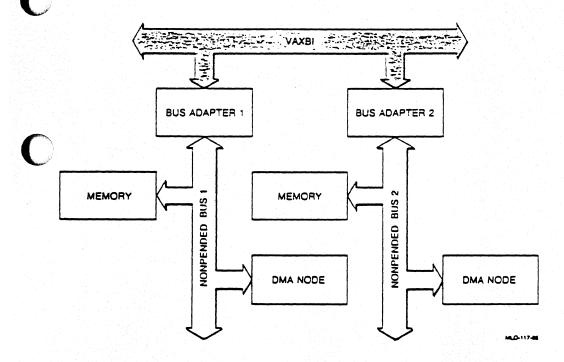
Figure AN5-3: Configuration with Two Nonpended Buses
