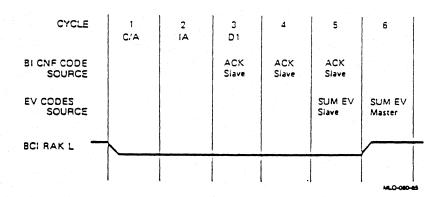
Figure 15-3: Summary EV Code Timing for Successful Write-Type and BDCST Transactions (Longword Write)
