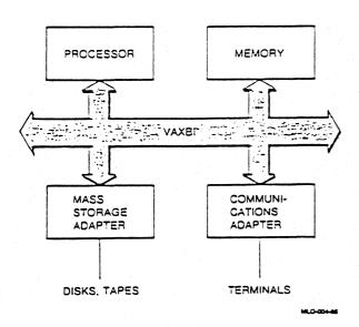
Figure 1-4: Small System Configuration with One Processor
