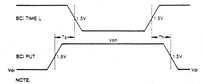
BCI input signals should have rise and fall times of < 5 ns (between 0.8 and 2.0 volt points).
