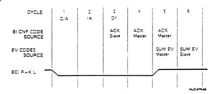
Figure 15-4: Summary EV Code Timing for Successful Read-Type Transactions (Longword Read)
