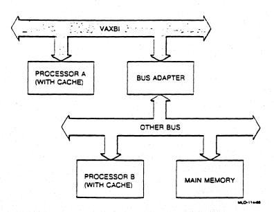
Figure AN2-3: Configuration with Multiple Buses
