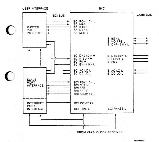
Figure 1-3: Block Diagram of VAXBI Node
