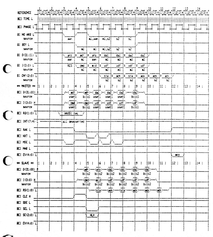
Figure 21-11: Octaword WMCI with Variable STALLs for Each Longword of Data
