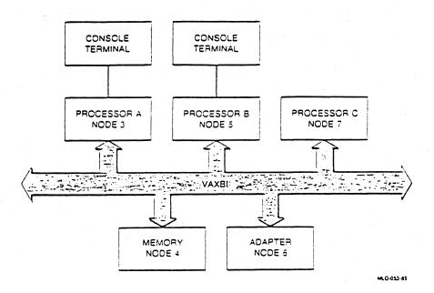
Figure 9-1: Console Configuration
