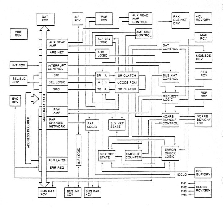
Figure 14-2: Block Diagram of the BIIC
