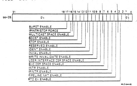
This register description makes reference to the BCI SEL L and BCI SC<2:0> L lines, which are described in Sections 15.5.4 and 15.5.5.
