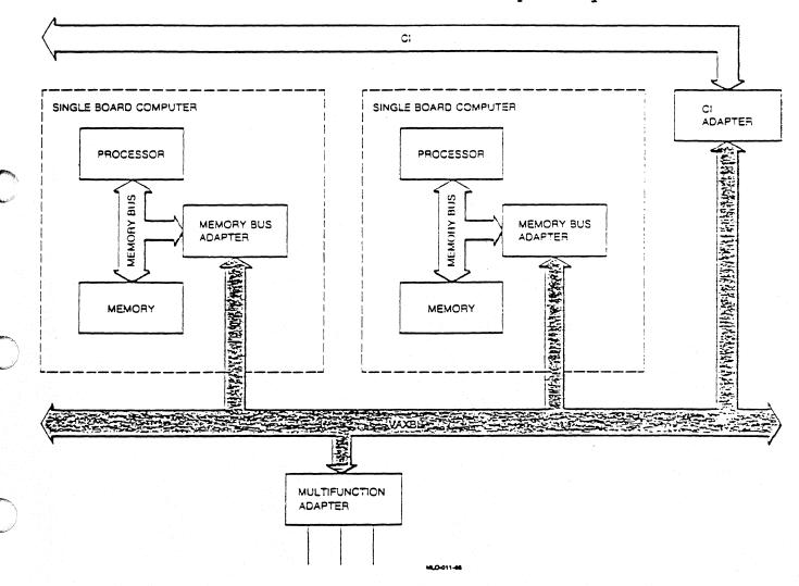
Figure 1-11: Configuration of a Cluster Node
