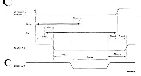
Figure 6-2: System Reset Timing Diagram
