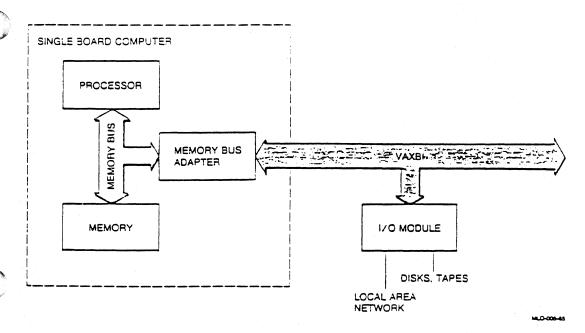
Figure 1-5: Stand-Alone Single Board Computer Configuration
