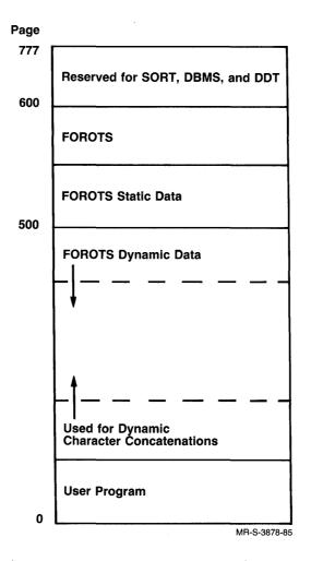
Figure 15-1: Run-time Memory Layout for Section Zero
