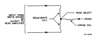
Figure 4-7 Simplified Read/Write Head Circuit
