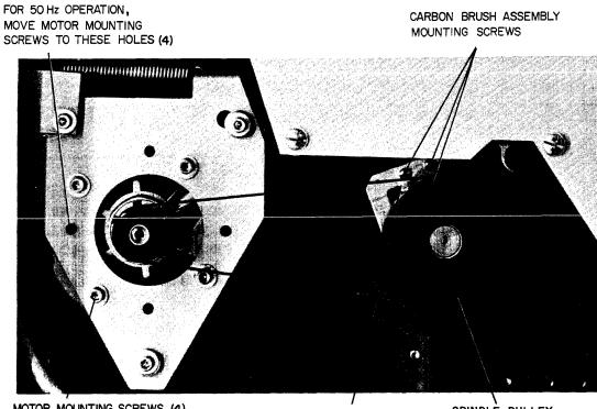
MOTOR MOUNTING SCREWS (4) (SHOWN FOR 60 Hz OPERATION)
