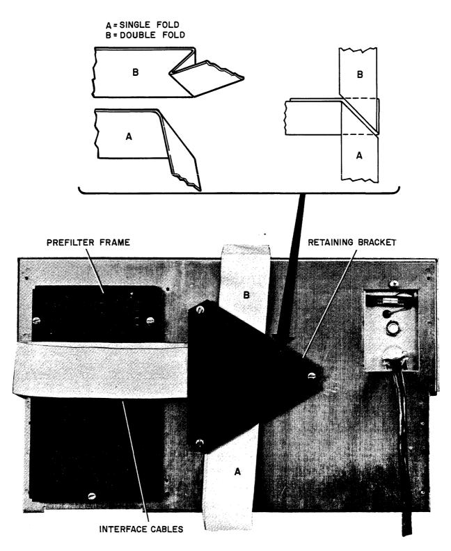
Figure 2-4 RK8/E Interface Cable Installation
