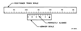
Figure 5-11 How to Read a Vernier
