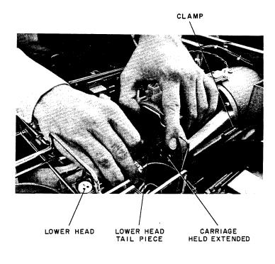
b. Lower Head Removal and Installation
