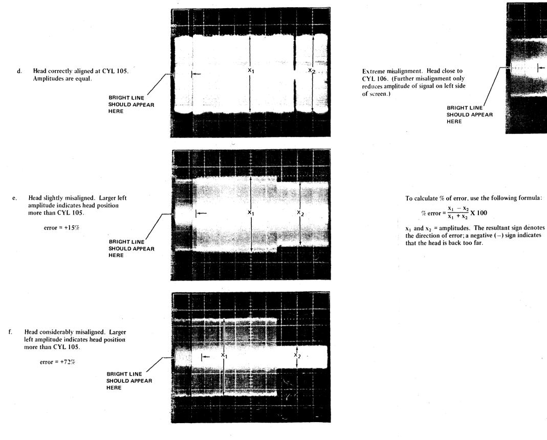
Figure 5-22 RK05K-AC Head Alignment Waveforms
