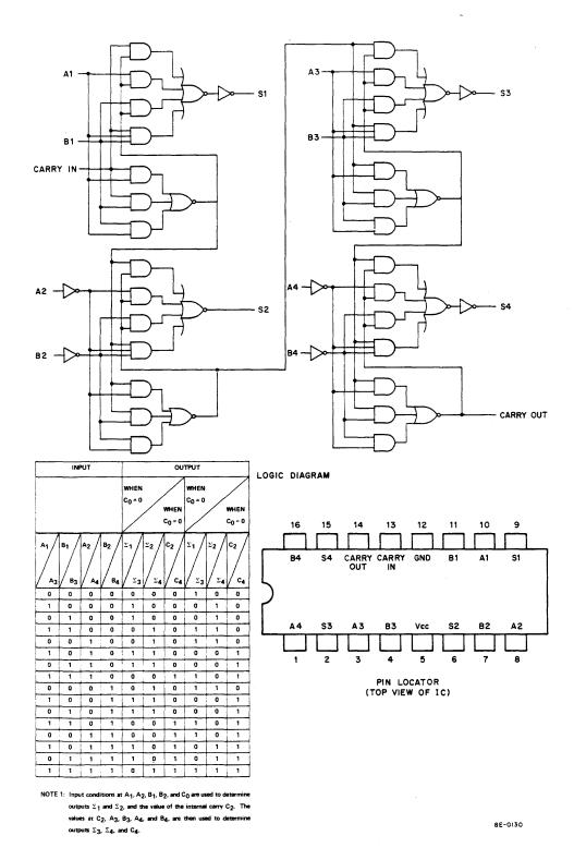
Figure E-2 7483 4-Bit Binary Full Adder
