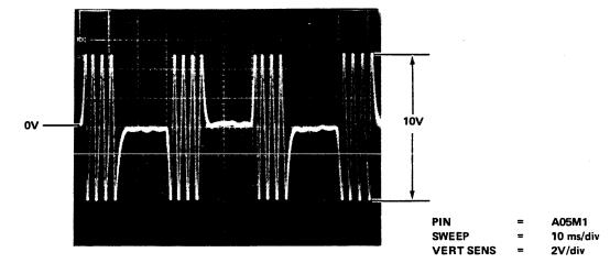
a. Correct Waveform (Symmetrical Signal)
