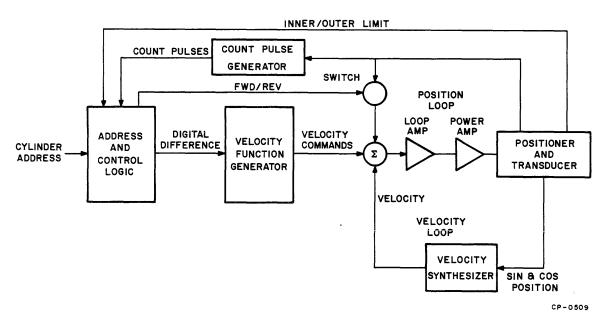
Figure 4-11 Servo System Block Diagram
