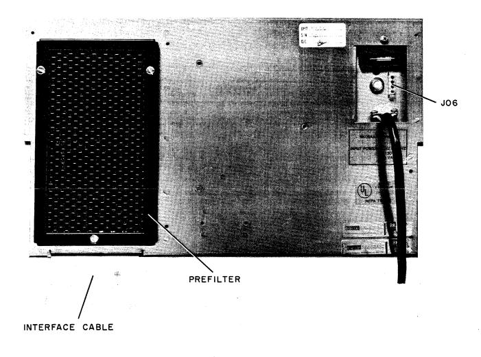
Figure 2-2 RK11C or RK11D Interface Cable Installation
