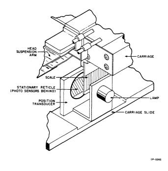
Figure 4-12 Linear Positioner Transducer
