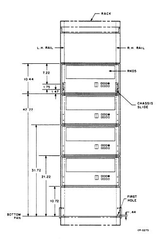
Figure 2-3 Chassis Slide Mounting
