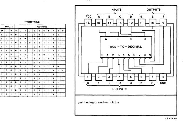
Figure E-6 74145 TTL MSI Lamp, Logic, or MOS Drivers
