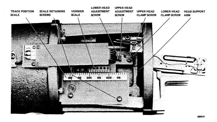
Figure 5-23 Read/Write Head Adjustments
