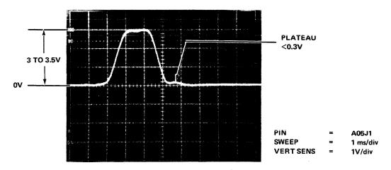
Figure 5-21 Outer Limit Waveform
