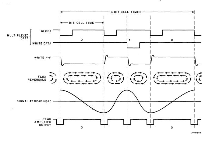
Figure 4-8 Double Frequency Pulse Relationship
