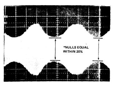
Extreme misalignment. Head close to CYL 106. (Further misalignment only reduces amplitude of peak.)
