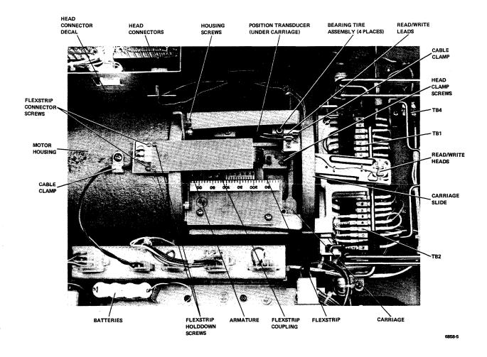
Figure 5-4 Top View of RK05 with Cover Removed
