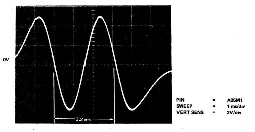
Figure 5-17 Velocity Amplitude Waveform
