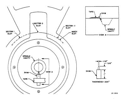
Figure 5-14 CE Test Cartridge Shim Installation
