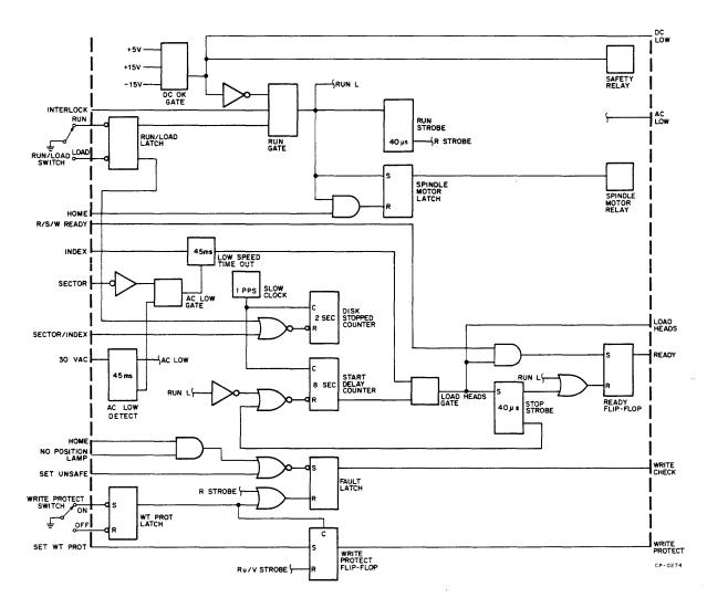
Figure 4-9 Control and Interlock Block Diagram
