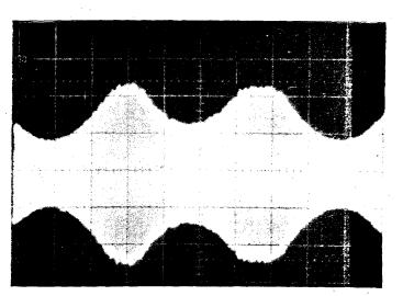
Head correctly aligned at CYL 105. Null amplitudes are equal. d.
