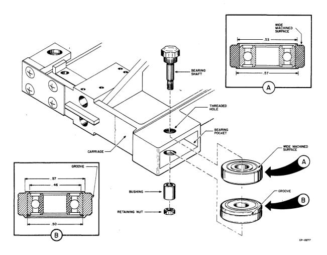
Figure 5-5 Carriage Bearing Assembly Removal
