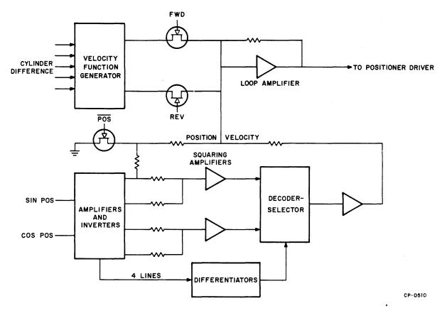
Figure 4-13 Simplified Positioner Servo Logic
