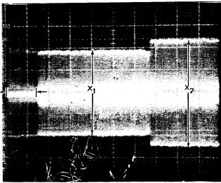
d. Head correctly aligned at CYL 105. Amplitudes are equal.
