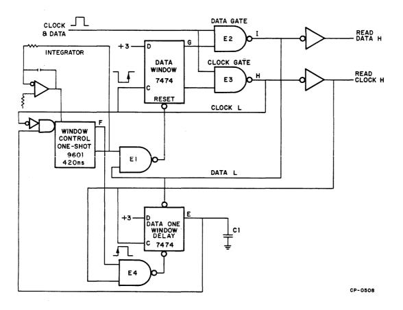
Figure 4-15 Simplified Data Separator Circuit
