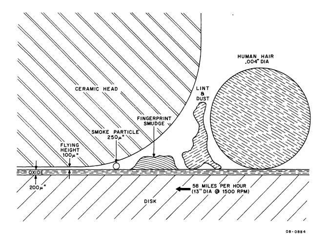
Figure 1-8 Relationship of Disk Head, Disk, and Contaminants
