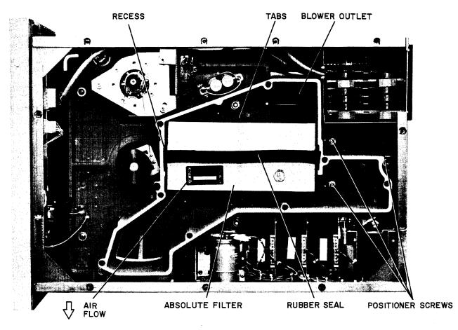
Figure 5-2 Absolute Filter Removal
