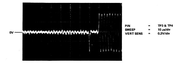
Figure 5-25 Index/Sector Waveform
