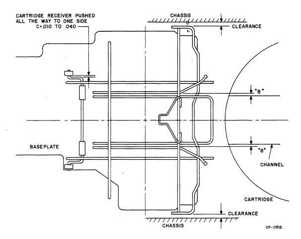
Figure 5-27 Cartridge Receiver Clearances
