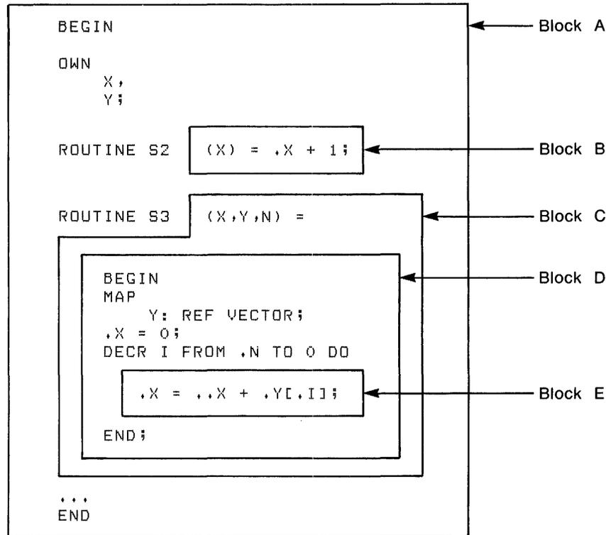
The blocks in this example are labeled in the same way as in the previous example. Three of the blocks are implicit; that is, they are assumed to exist even though a BEGIN-END or parenthesis pair is not used. Specifically, Blocks B and C are the implicit blocks that each surround the formal-names and the routine-body of a routine-declaration. Block E is the implicit block that surrounds the body of a loop.
