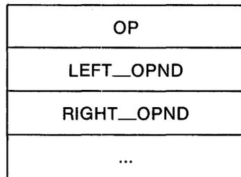
The op field is used to contain a code for the kind of arithmetic operator represented, and the LEFT\_OPND and RIGHT\_OPND fields are used to contain addresses of other such nodes.
