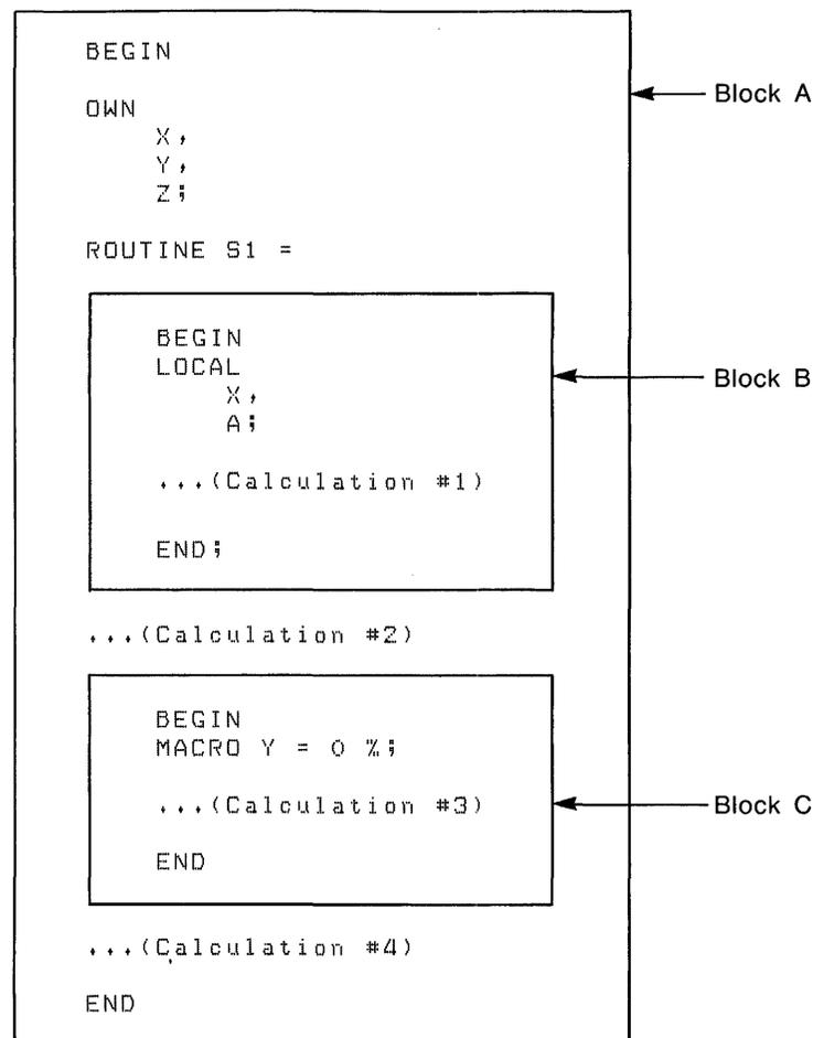
The three blocks in this example are enclosed in boxes that are identified as A, B, and C for convenience of discussion. Block A designates the entire example (including the contents of Block B and Block C). The details of the calculations performed by the example block are not important, so they are omitted. The places where names could be used in calculations are called Calculation #1, Calculation #2, and so on.
