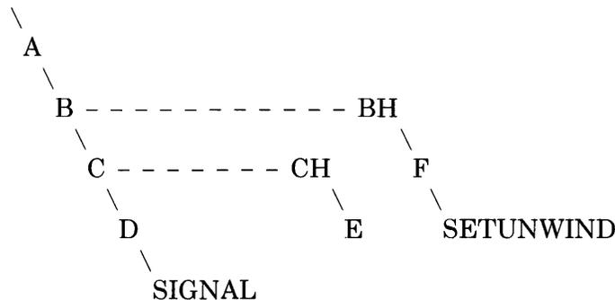
In this diagram, a diagonal line indicates that the upper routine calls the lower routine, e.g., A calls B, B calls C, and so on. A horizontal line indicates
