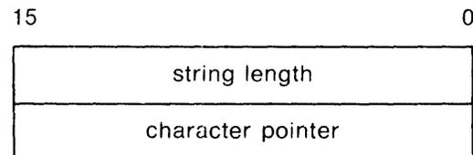
This format follows the PDP-11 Extended Instruction Set guidelines. Note that the “string length” must be an unsigned 16-bit quantity in the range 0 to 65535 decimal.
