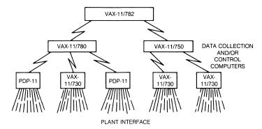
Figure 6-5 • Typical Manufacturing Network
