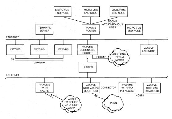
Figure 6-8 • Sample DECnet Phase IV Configuration
