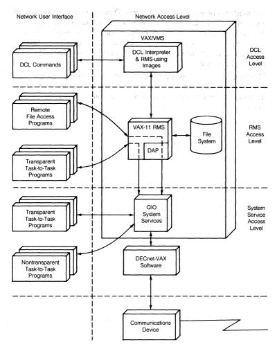
Figure 6-12 • Network Access Levels and DECnet-VAX User Interface
