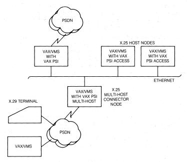
Figure 6-11 • DECnet Network Configuration Showing Examples of X.25
