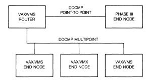
Figure 6-9 • Typical DDCMP Point-To-Point Connections
