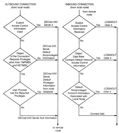
Figure 6-7 • Access Control For Inbound Connections
