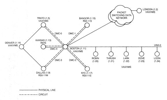
Figure 6-1 • Typical Single-Area DECnet Network
