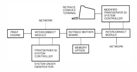
Figure 1 RETrACE Analysis System Hardware
