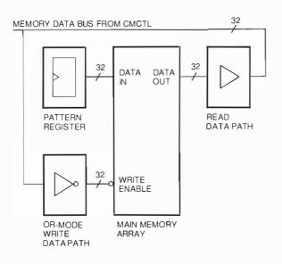
Figure 2 OR-mode Circuit
