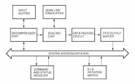
Figure 4 Block Diagram of DECimage 1200 Accelerator Hardware
