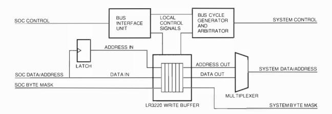
Figure 5 Write Buffer
