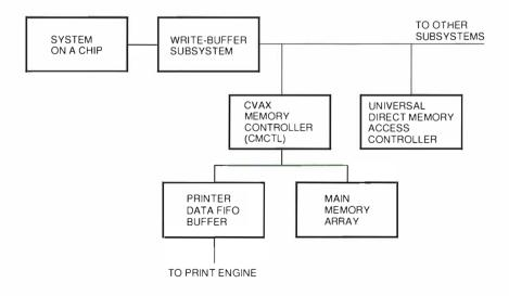
Figure 4 Interconnection of Turbo Controller Subsystems
