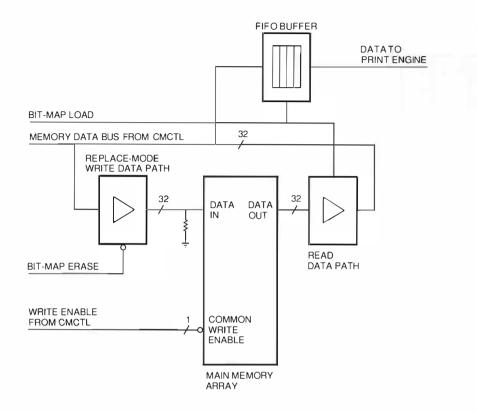
Figure 3 Scan-erase Circuit
