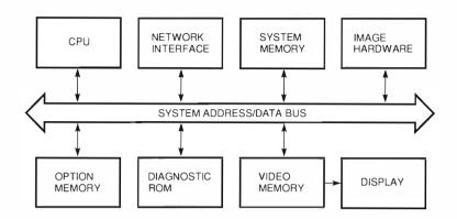
Figure 3 VT1200 System Architecture
