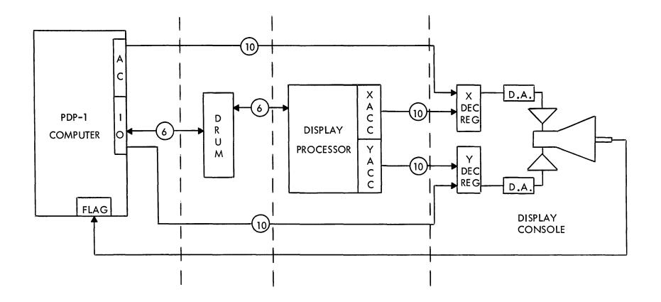
Figure 1 Display System Block Diagram
