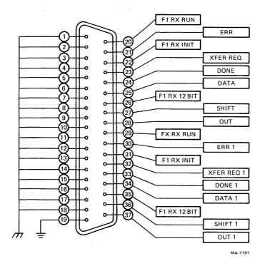
Figure F-2 RX278 Floppy Drive Interface Connector
