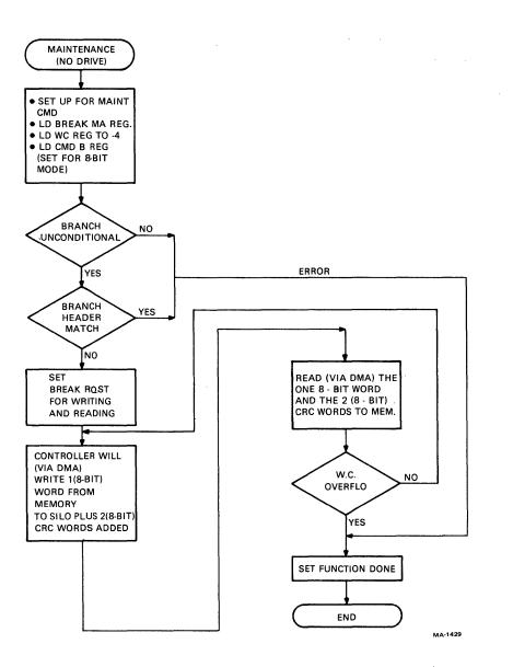
Figure 7-6 Maintenance Command, Operational Sequence
