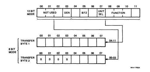
Figure 5-1 RX278 Diskette Subsystem Instruction Format
