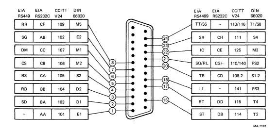
Figure F-3 DP278 Communications Options Connector (Port0/Port 1)
