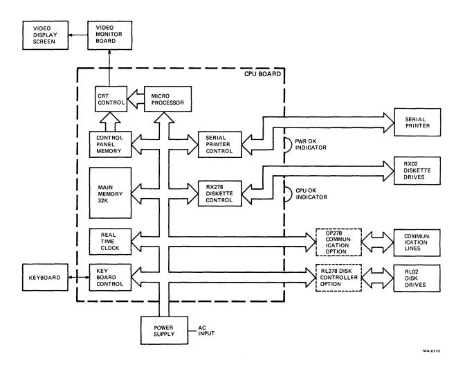
Figure 2-1 DECmate Block Diagram
