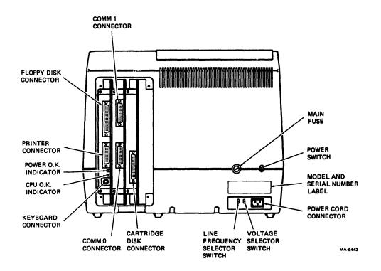
Figure 3-2 VT278 Rear Panel With I/O Cover Removed
