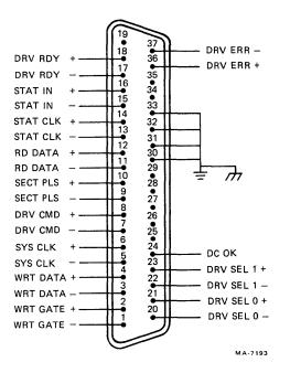
Figure F-4 RL278 Disk Cartridge Interface Connector
