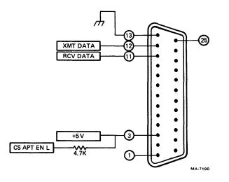
Figure F-1 VT278 Printer Port Connector
