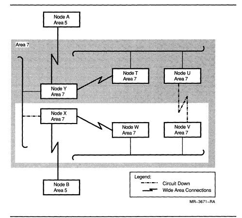
Figure 5–4 shows how an area that lacks redundant paths can become partitioned if one or more circuits fail.
