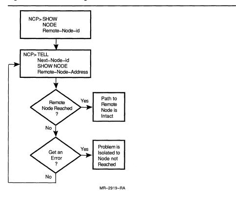
Figure 4-1 shows the routing path trace procedure in flowchart form.
