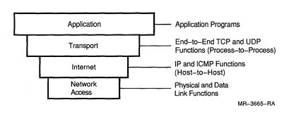
The Internet Protocol model specifies the functional layers of TCP/IP software on each host, and the communications protocols through which the corresponding layers at different hosts communicate with each other. Each protocol is a set of messages with specific formats and rules for exchanging the messages. These protocols govern the operation of a communications link without regard to hardware.
