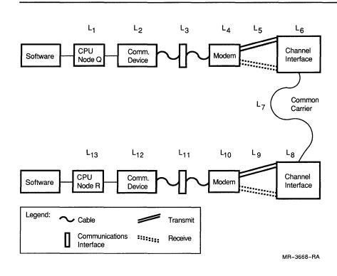
Figure 4–2 Components and Points of Loopback Testing
