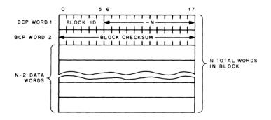
Figure 5-4 Block Format, File-Structured Mode
