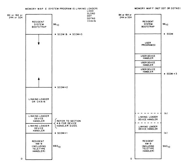
The System Loader learns which I/O handlers are required by the Linking Loader, loads them relocatably and then loads the Linking Loader relocatably.
