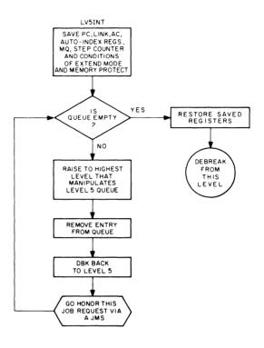
Figure 7-1 Structure of API Software Level Handler
