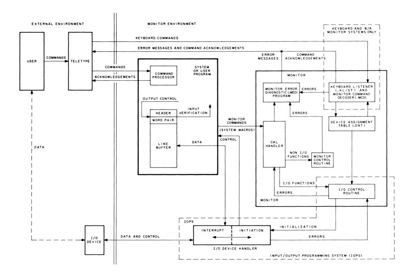
Figure 2-2 Command, Control, and Data Flow in Monitor Environment
