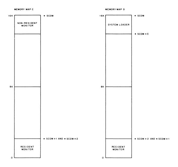
The resident Monitor loads the non-resident Monitor (via the resident system device handler) into upper core, overlaying the System Bootstrap To load a user FOREGROUND program, the non-resident Monitor brings in the System Loader, overlaying itself. For FOREGROUND loading, the System Loader is the Linking Loader.
