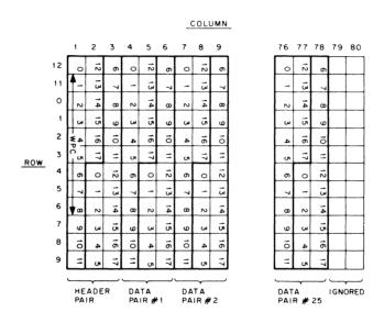
Figure 7-2 IOPS Binary Input Card Format
