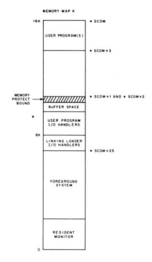
The .EXIT from the Linking Loader causes the user program I/O handlers to be block transferred to their running position, the memory protect bound to be set just above the buffer space, and control given to the user program.
