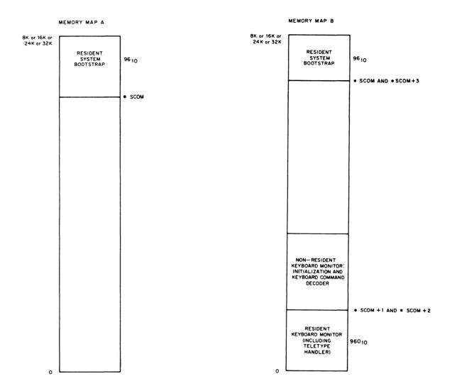
The System Bootstrap is loaded via the paper tape reader in HRM mode.
