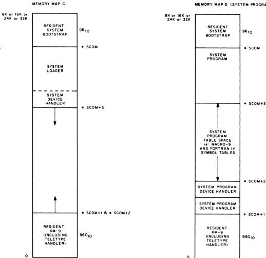
The Keyboard Monitor loads (DUMP mode) the System Loader and the system device handler from the system device
