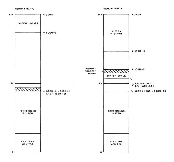
When a keyboard command requests loading of a BACKGROUND system or user program, the non-resident Monitor brings in the System Loader, overlaying itself.
