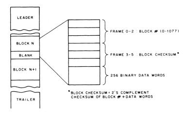
Figure 5-3 Paper Tape Block Format
