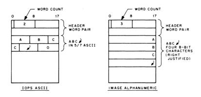
Figure 2-9 IOPS ASCII and Image Alphanumeric
