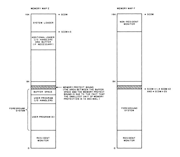
The System Loader first loads any additional I/O handlers required for loading. It then loads the user program and the I/O handlers that it requires, and allocates buffer space.
