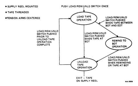
Figure 4-2 Load Switch State Diagram
