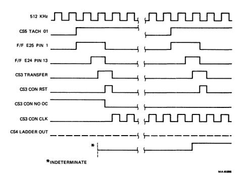
Figure 6-15 Capstan Timing Diagram
