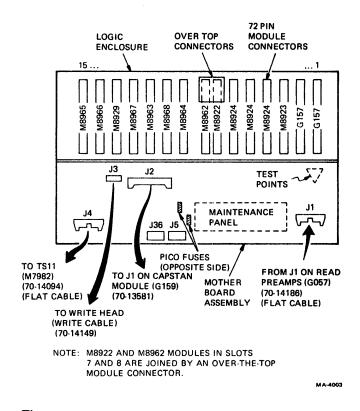
Figure 7-22 Logic Rack (Rear View)
