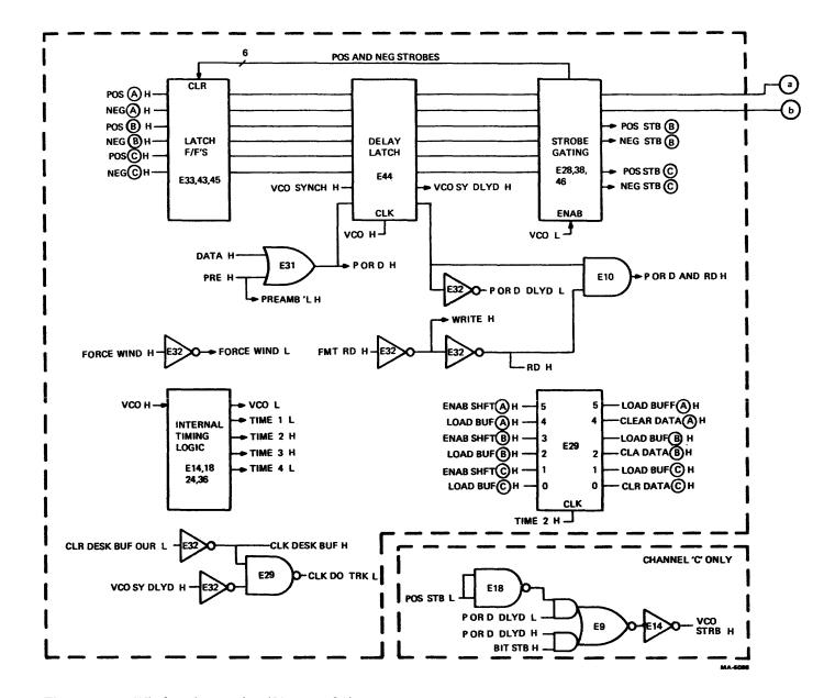
Figure 6-31 Window Generation (Sheet 1 of 2)
