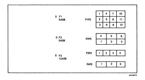
Figure 7-7 Power Supply Mate-N-Lok Connector Layout
