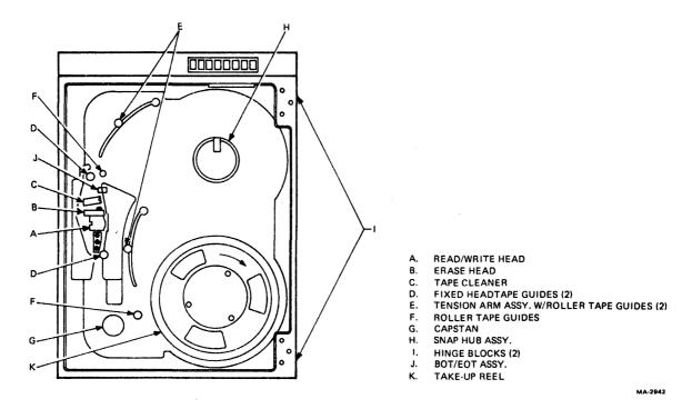
Figure 3-1 Transport Components to Clean
