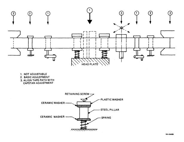
Figure 7-12 Tape Path Alignment
