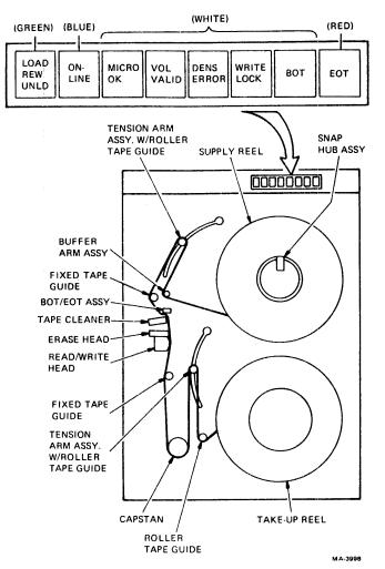
Figure 1-3 Transport Assemblies (Front View)
