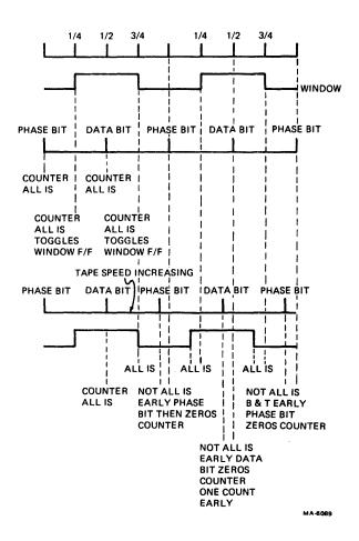
Figure 6-34 Window Adjustment
