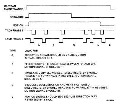
Figure 7-5 Capstan Simulated Motion Waveforms
