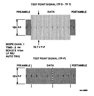
Figure 7-20 Read Preamplifier Adjustment
