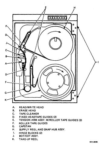
Figure 6-24 Tape Loading Path
