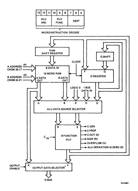
Figure 6-4 2901 Microprocessor Slice
