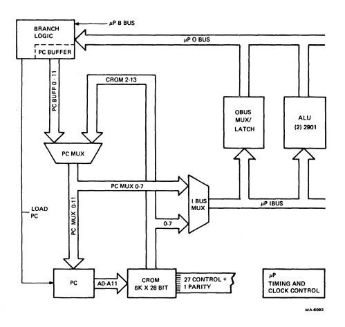
Figure 6-3 Microprocessor Block Diagram
