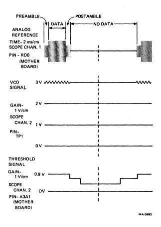
Figure 7-21 VCO and Threshold Waveforms
