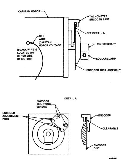
Figure 7-16 Capstan Tachometer Encoder Assembly
