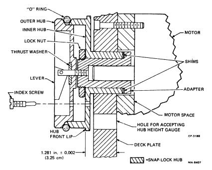
Figure 7-9 Snap Lock Hub Cross Section
