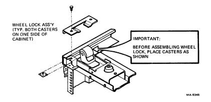
Figure 2-8 Caster Lock Assembly
