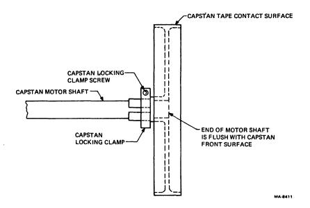
Figure 7-13 Capstan Positioning on Capstan Motor Shaft
