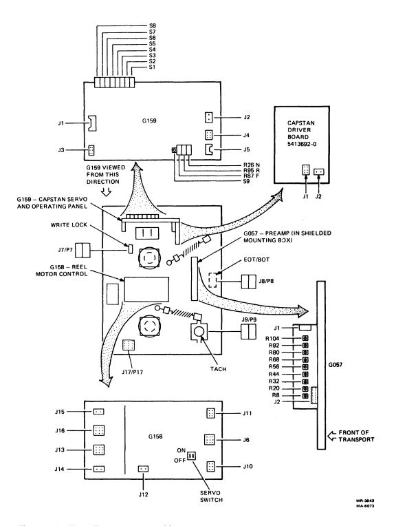
Figure 6-2 Tape Transport Assembly
