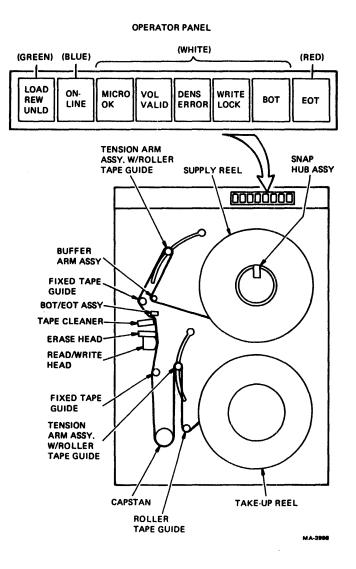
Figure 7-2 Transport Assemblies (Front View)
