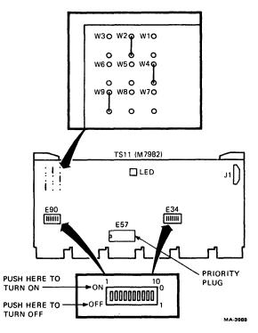
Figure 2-12 M7982 Interface Module
