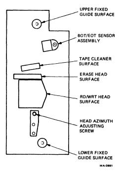
Figure 7-15 BOT/EOT Sensor and Head Skew Adjustment
