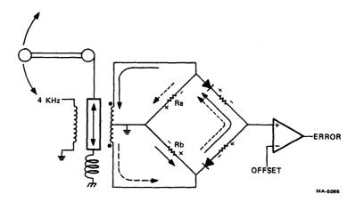
Figure 6-22 Tension Arm Transducer
