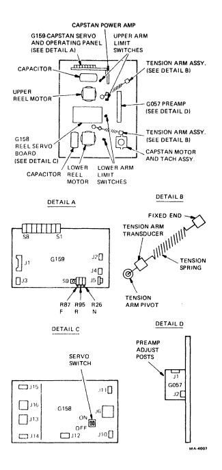
Figure 1-4 Transport Assemblies (Rear View)
