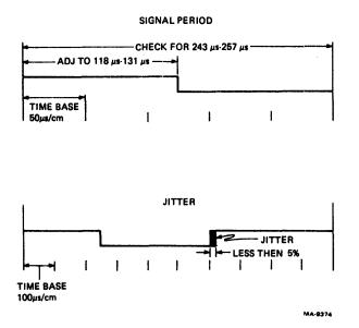
Figure 7-18 Capstan Speed Adjustment
