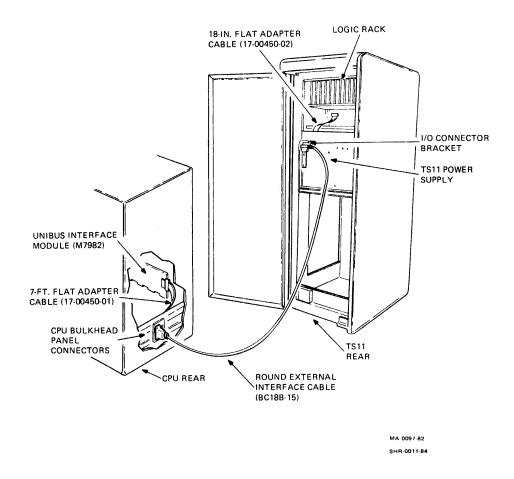
Figure 2-13 TS11 Signal Cabling
