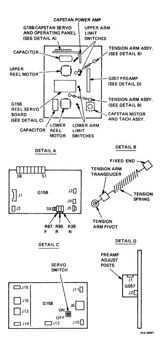
Figure 7-3 Transport Assemblies (Rear View)
