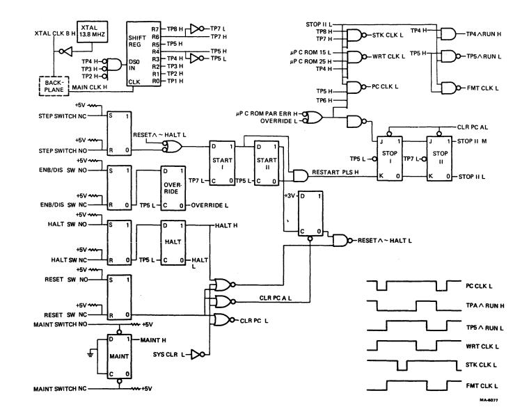
Figure 6-7 Clock Generator and Control Logic
