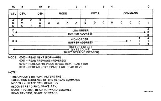
Figure 5-9 Read Command Packet Example
