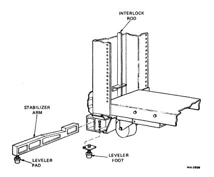
Figure 2-7 H9602 Stabilizer Leg and Leveler Feet Locations
