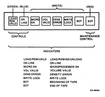
Figure 4-1 TS11 Transport Controls and Indicators
