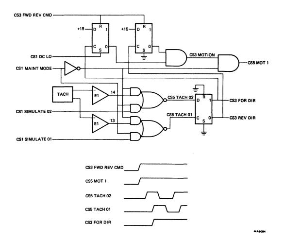
Figure 6-13 Motion and Direction Detection
