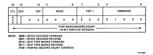
Figure 5-12 Position Command Packet Example
