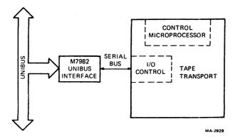
Figure 1-1 TS11 Subsystem Configuration
