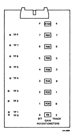
Figure 7-19 Read Preamplifier Locator
