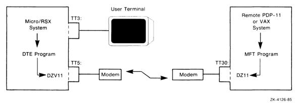
Figure 9-2 Terminal Emulation with a Remote System
