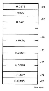
Figure 19-2: Format of Pool Header Area
