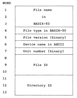
Figure A-1 PRT Send Data Buffer Format
