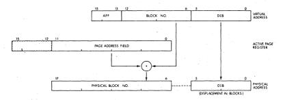
Figure 8-10 Construction of a Physical Address
