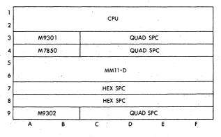
Figure 7-2 16K Core using MM11-D
