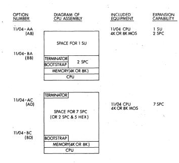
Figure 6-1 PDP-11/04 CPU Diagrams
