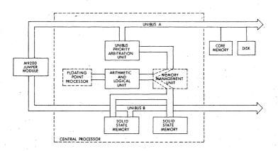
Figure 9-1 PDP-11/55, PDP-11/45 System Block Diagram
