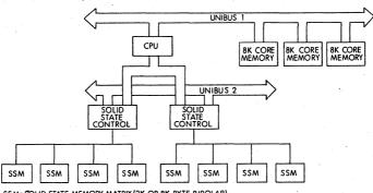
SSM= SOLID STATE MEMORY MATRIX (2K OR 8K BYTE BIPOLAR)
