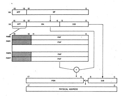
Figure 10-4 Construction of a Physical Address
