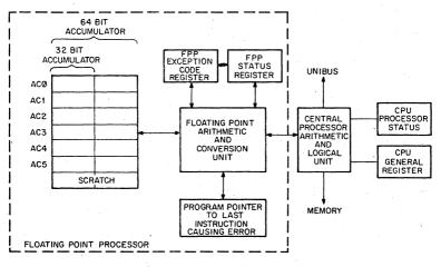
Figure 11.1 Floating Point Processor
