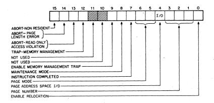
Figure 10-8 Format of Status Register #0 (SR0)
