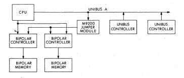
4. The two MS11 solid state memory controls are connected to a single UNIBUS (UNIBUS-B) that can be easily separated from the 11/45 CPU UNIBUS (UNIBUS-A) by removing a simple jumper module (M9200), thus facilitating dual UNIBUS systems. UNIBUS B does not have its own Unibus arbitration control logic; thus, a second PDP-11 CPU is required for other than NPR transfers from a single device.
