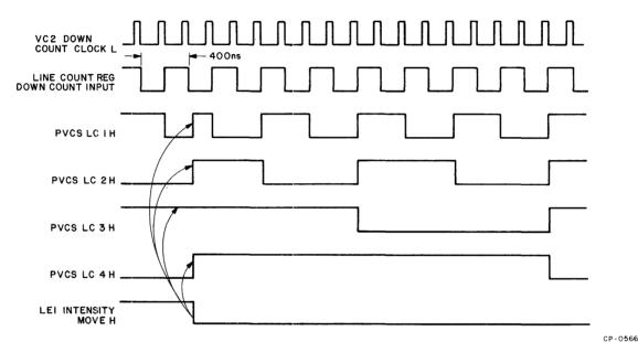
Figure 2-15 Line Count Register, Timing Diagram
