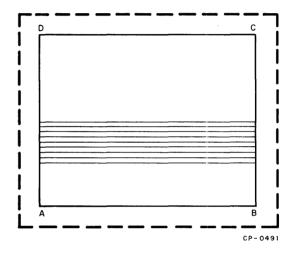
Figure 3-17 Vertical Phosphor Display Pattern
