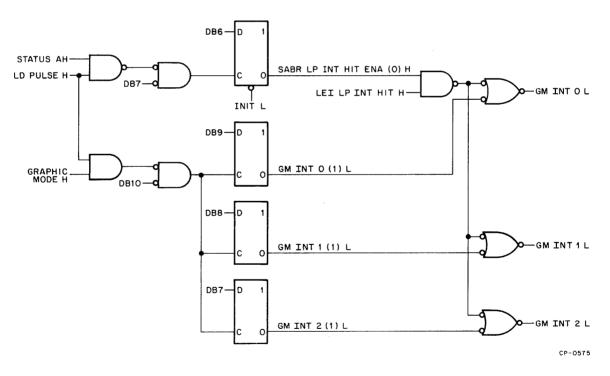
Figure 2-10 M7013 Intensity Level Control
