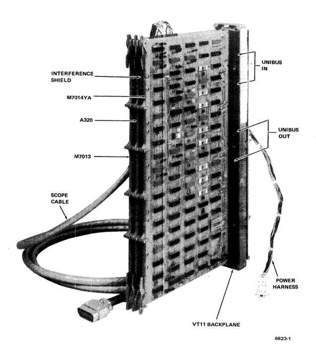
Figure 1-2 VT11 Graphic Display Processor
