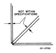
Figure 3-10 Faulty Box with X Display
