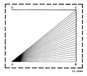
Figure 3-14 Horizontal Vector Length Display Pattern
