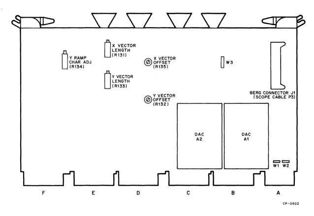
Figure 3-1 Adjustment Locations, A320 Module
