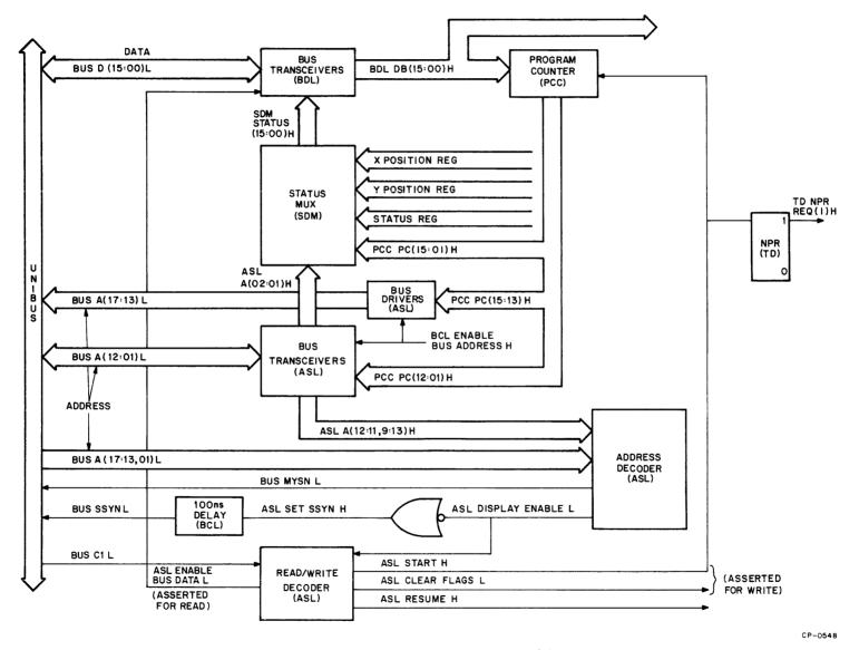
Figure 2-1 Unibus Address and Data, Block Diagram
