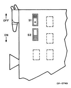
Figure 3-5 Maintenance Switches, M7013 Module
