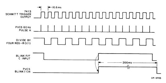
Figure 2-16 Blink Timing Diagram
