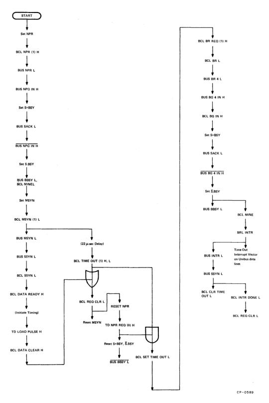
Figure 2-4 NPR/Time Out Interrupt, Flow Diagram
