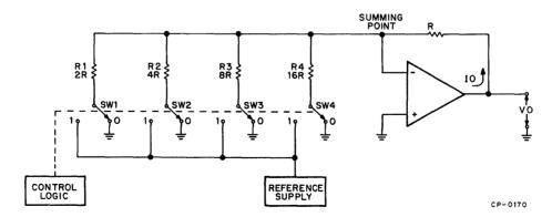
Figure 2-45 Typical Current Summing Ladder
