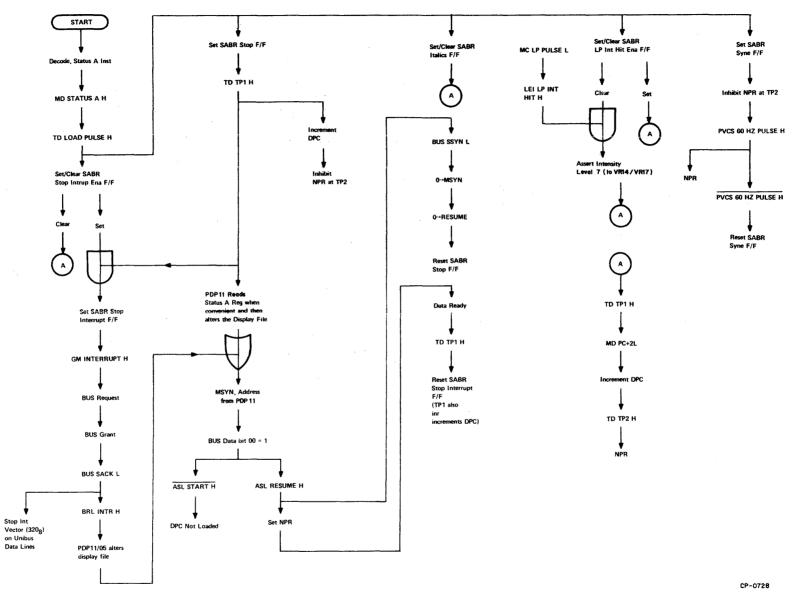
Figure 2-9 Status A Instruction Flow Diagram
