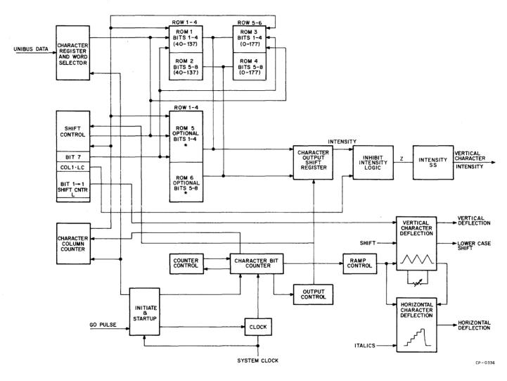
Figure 2-29 Character Generator, Block Diagram
