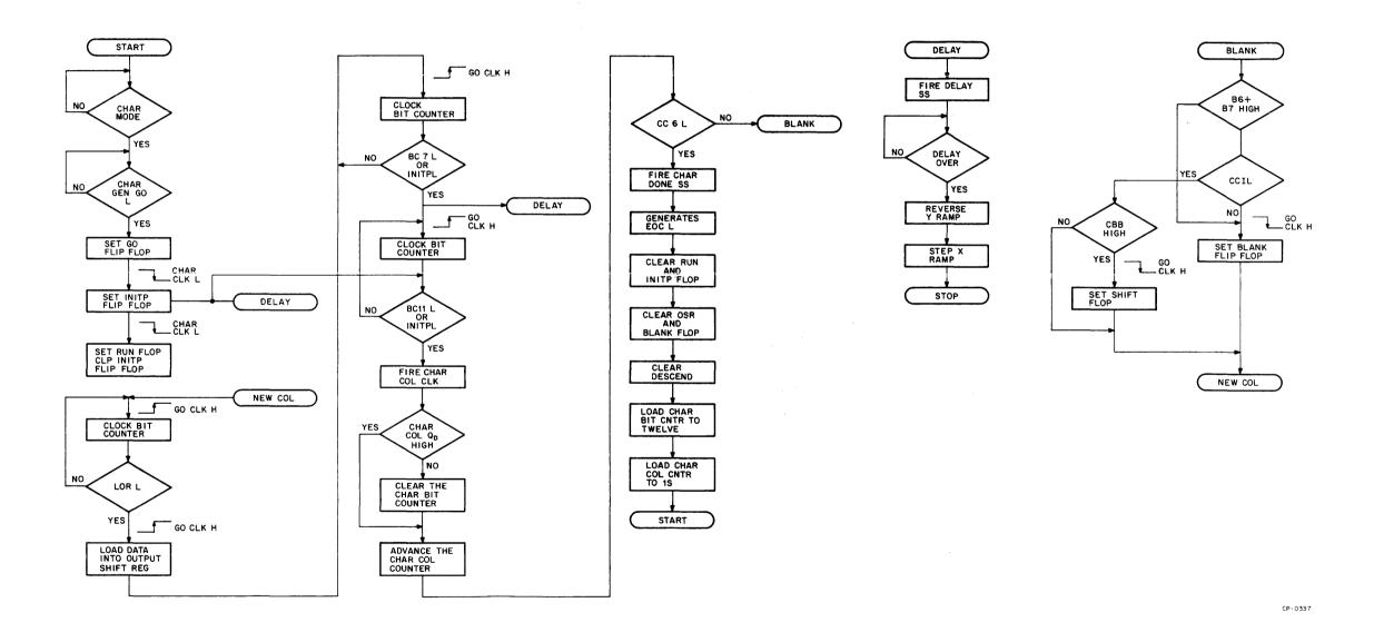
Figure 2-30 Character Generator, Flow Diagram
