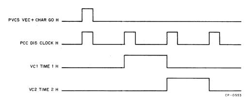
Figure 2-38 Time Shift Register, Timing Diagram (M7014YA-VC1)
