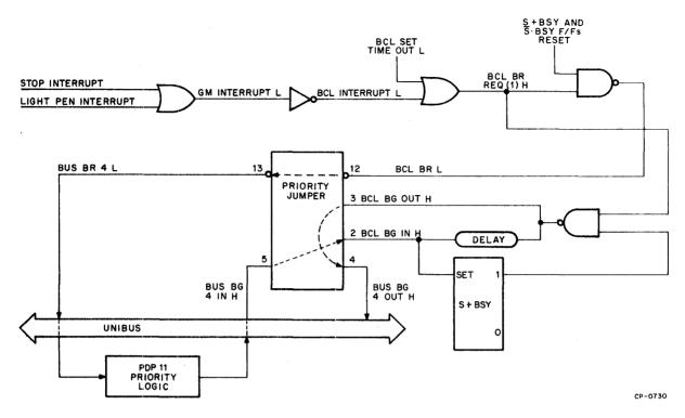
Figure 2-5 Bus Request and Bus Grant, M7014YA Module
