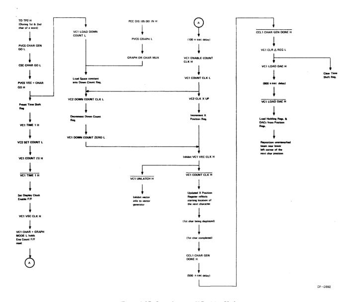
Figure 2-37 Intercharacter X Position Update, Flow Diagram
