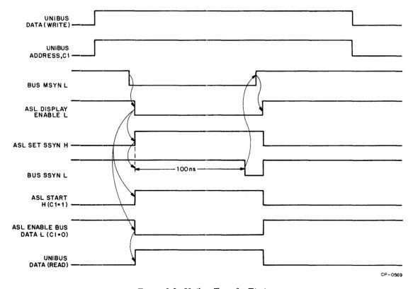
Figure 2-2 Unibus Transfer Timing
