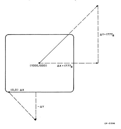
Figure 2-22 Cut-Off Vector Displays
