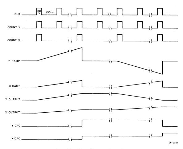
Figure 2-25 Vector Generator, Timing Diagram
