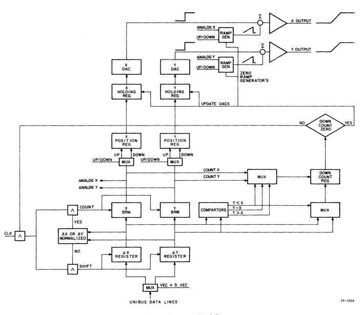
Figure 2-23 Vector Generator, Block Diagram
