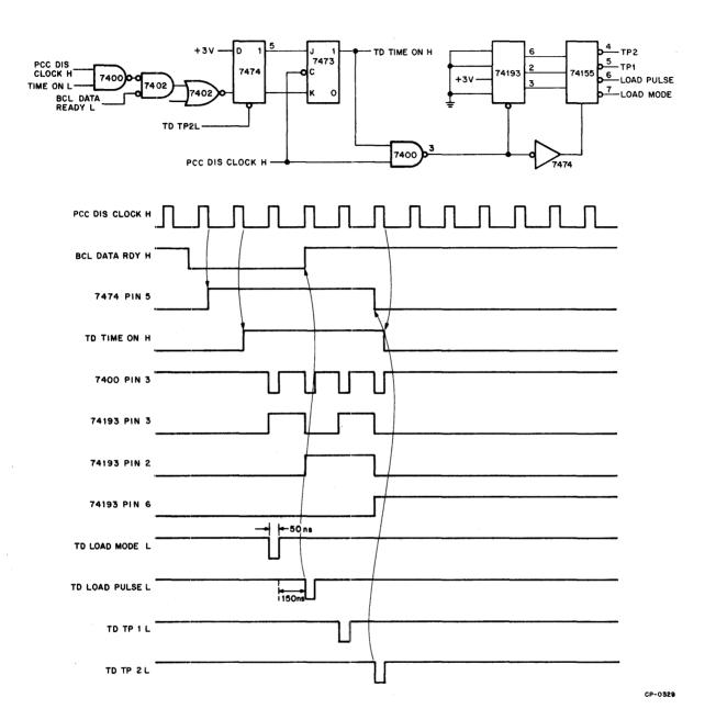
Figure 2-6 Display Processor Timing Diagram – M7013 Module
