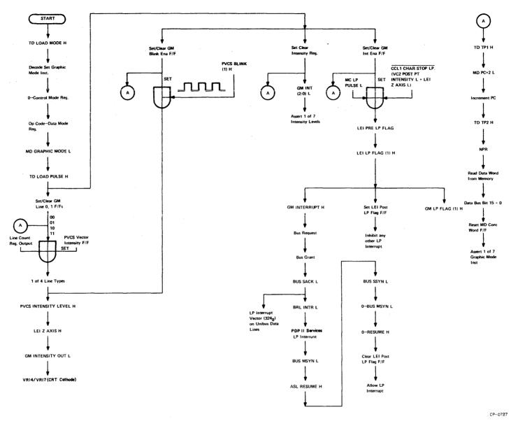
Figure 2-14 Set Graphic Mode Instruction Flow Diagram
