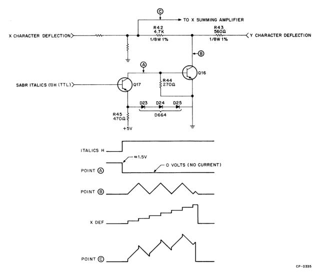
Figure 2-43 Italics Control Circuit
