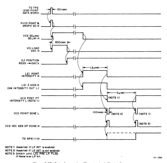
Figure 2-27 Point Instruction (Termination), Timing Diagram
