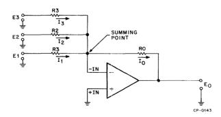
Figure 2-46 Summing Amplifier Configuration
