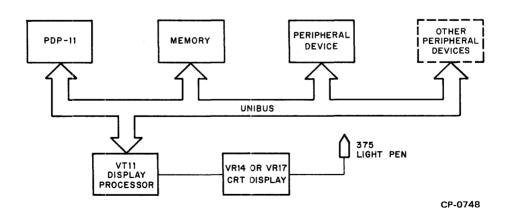
Figure 1-1 VT11 Graphic Display Processor in System Configuration
