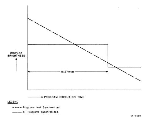
Figure 2-11 Relationship of CRT Brightness to Program Length
