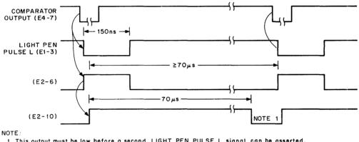
1. This output must be low before a second LIGHT PEN PULSE L signal can be asserted.
