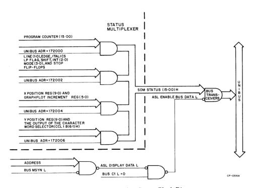
Figure 2-3 Reading Status, Block Diagram
