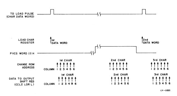
Figure 2-34 Word Selection and ROM Addressing, Timing Diagram
