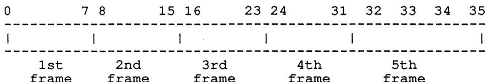
For each data word in memory, there are five magnetic tape bytes per 36-bit word, with parity bits unavailable to the user. Bits are read and written on the tape as shown below.
