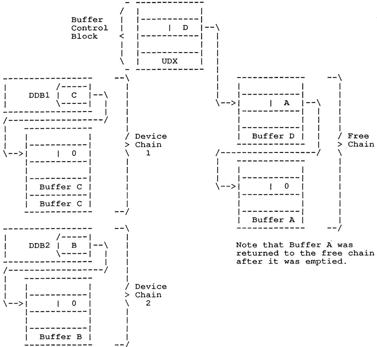
**Figure 11-7: One Buffer Moved Back to Free Chain**
