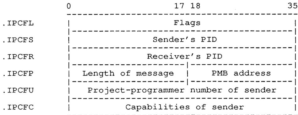
Figure 7-1: Packet Header Block
