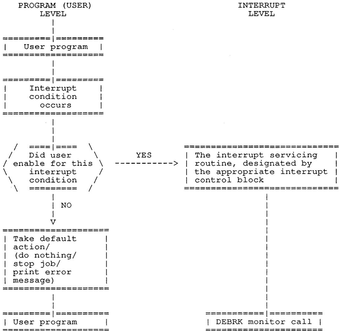
Figure 6-1: The Software Interrupt Process
