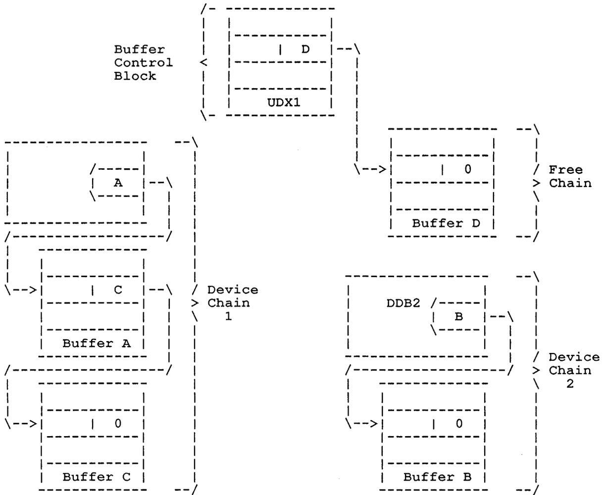
Figure 11-6: Multiple Buffers in Multiple Device Chains
