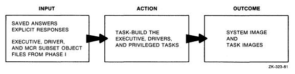
Figure 5-1 Logical Flow of SYSGEN Phase II
