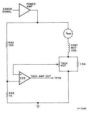
Figure 4-12 Tachometer Circuit
