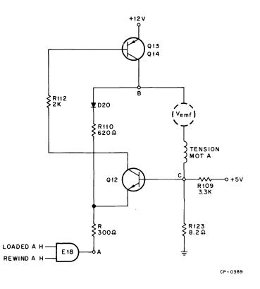
Figure 4-13 Rewind Control Circuit
