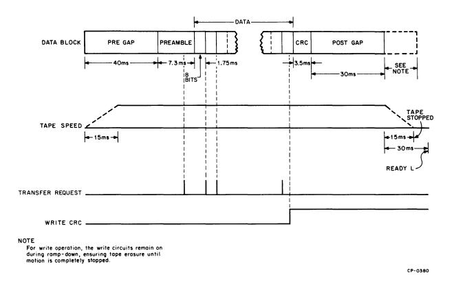
Figure 4-4 Write Data Block
