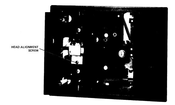
Figure 5-7 Head Skew Adjustment
