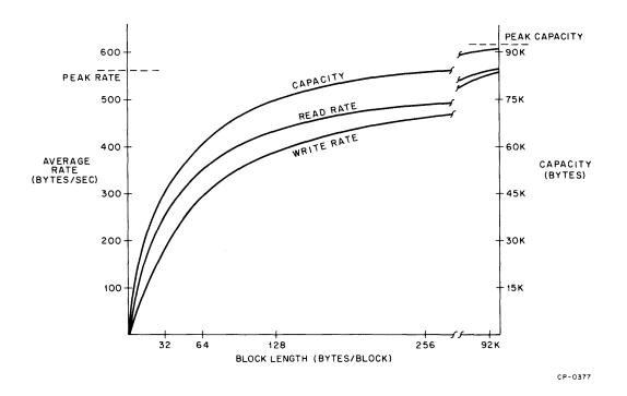
Figure 1-1 Capacity and Data Rate vs Block Length
