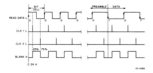
Figure 4-9 Simplified Blank H and Read Clock Timing
