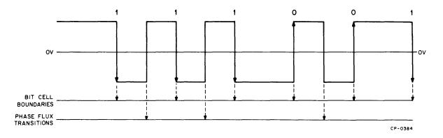
Figure 4-7 Typical Phase Encoded Waveform
