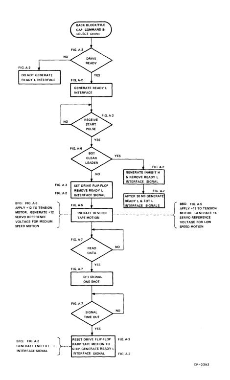
Figure 4-3 Back Block/File Gap Flow Chart
