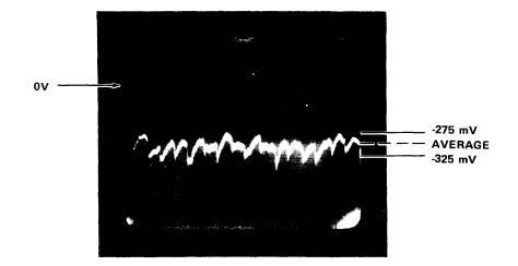
Figure 5-2 Control Motor Solenoid Adjustment
