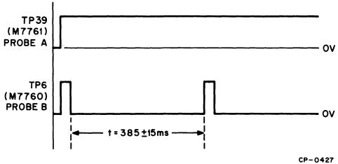
6. Adjust R24 (Pot C) on the M7760 module until t equals  $385 \pm 15$  ms.
