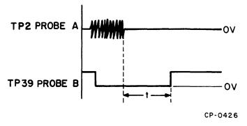
Figure 5-12 Signal Time Waveform
