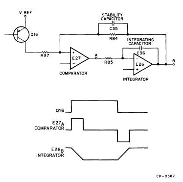
A-5). The resultant positive ramp signal from the integrator is then fed back to the positive comparator input, thereby equalizing the negative and positive comparator inputs.
