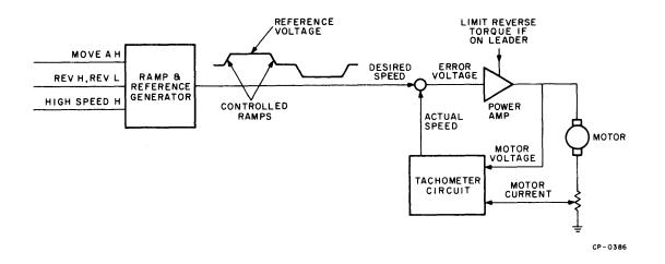
Figure 4-11 Simplified Control Motor Servo System
