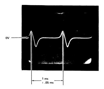
Figure 5-5 Fine Speed Adjustment
