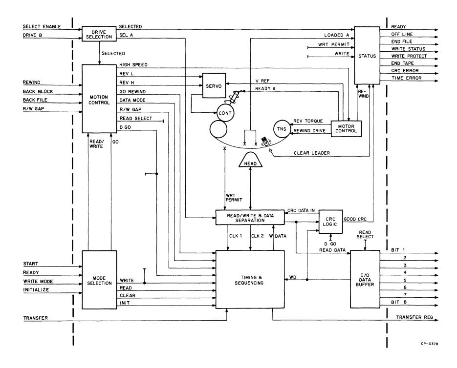
Figure A-1 Functional Block Diagram
