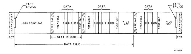
Figure 4-1 Typical Tape Format
