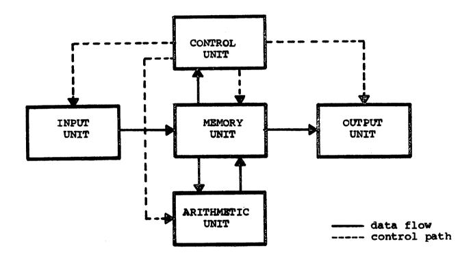
Figure 1-3 Basic Computer Block Diagram
