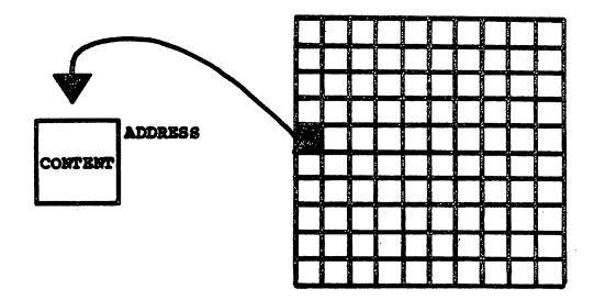
Figure 3-2 Conceptual Computer Memory Section
