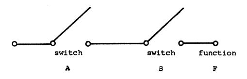
Figure 2-8 AND Circuit Diagram
