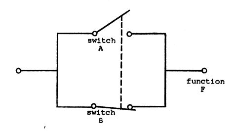
Figure 2-1Ø EXCLUSIVE OR Circuit Diagram
