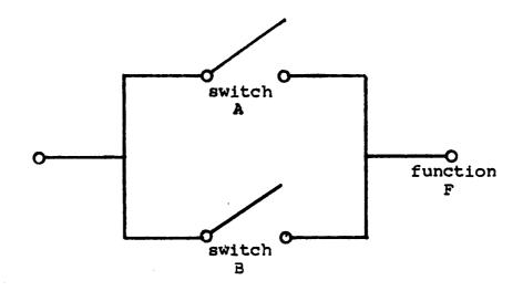
Figure 2-9 INCLUSIVE OR Circuit Diagram
