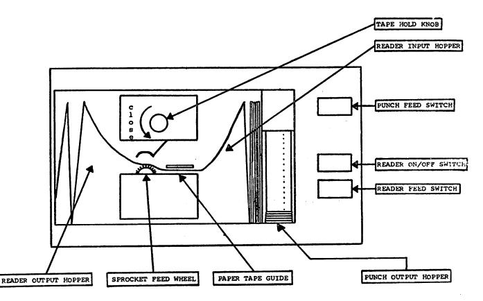
Figure 3-1Ø High Speed Reader and Punch
