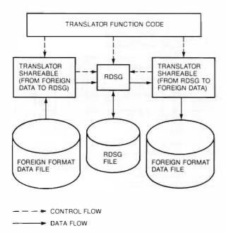
Figure 3 Data and Control Flow for Translation
