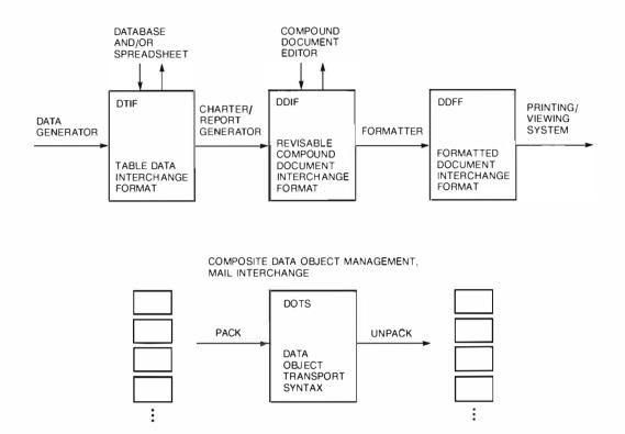
Figure 2 CDA Component Architectures
