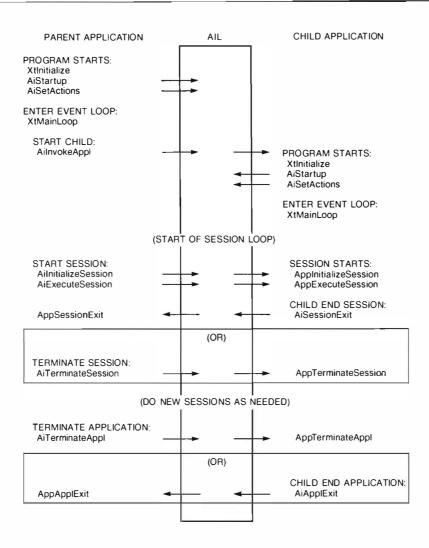
Figure 4 Basic AIL Routine Usage Sequence
