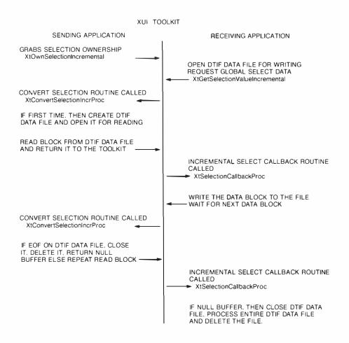
Figure 2 Incremental QuickCopy
