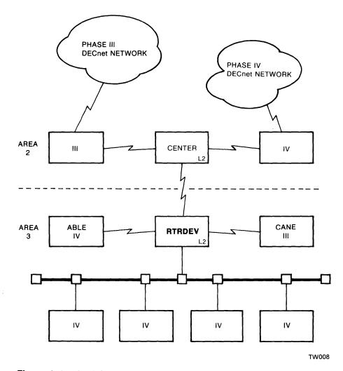
Figure 1–1: A DECnet Router Server with Three Point-to-point Lines
