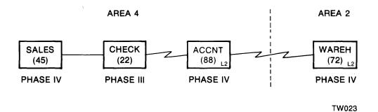
Figure 3–4: Improper Configuration of Phase III and Phase IV Nodes
