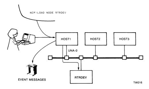
Figure 5–1: Using the LOAD Command
