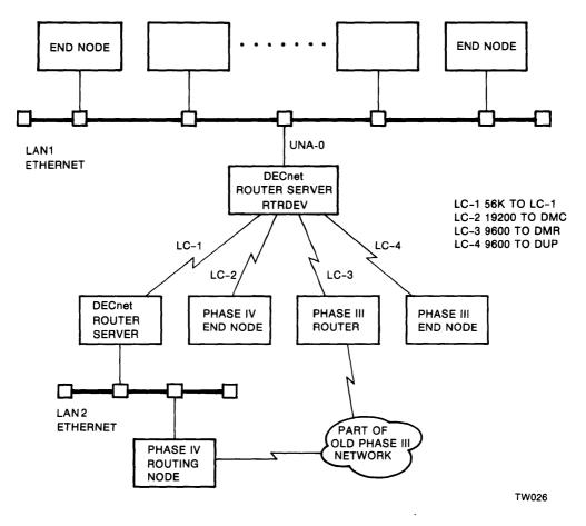
Figure 4–3: Configuration for Sample Customized Routing Configuration File
