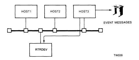
Figure 5–4: The TRIGGER Command: (3) First Host to Respond Loads the Server
