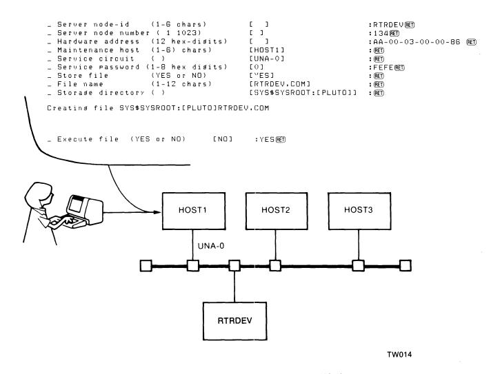
Figure 2–1: Setting up the DECnet Database for the Server on a VMS Host
