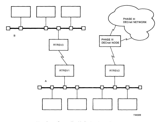
Figure 1–2: Two DECnet Router Servers Used in Conjunction on One Ethernet
