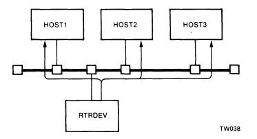
Figure 5-3: The TRIGGER Command: (2) Multicast Request-to-load Message
