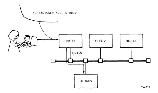
Figure 5-2: The TRIGGER Command: (1) Trigger Is Sent to the Server
