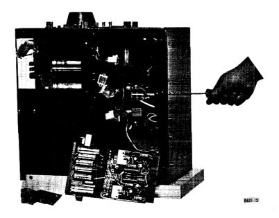
a. Remove the 7007165 as shown in Figure 4-4 and unscrew the four 6-32 heat sink mounting screws from the side chassis. Remove two pin connector from the high voltage bracket.
