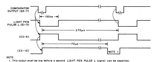
Figure 3-8 Light Pen Pulse Timing, G840 Module
