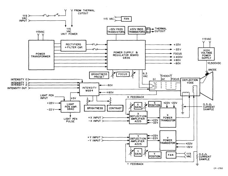
Figure 1-2 VR14L/VR17L Block Diagram
