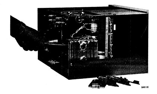
a. Remove circuit boards and the four 6-32 screws holding the deflection sink to the rear panel.
