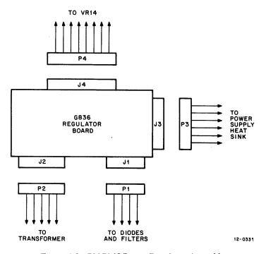
Figure 4-3 7007165 Power Regulator Assembly
