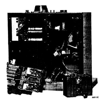
b. Lift heat sink straight out and repair faulty transistor.
