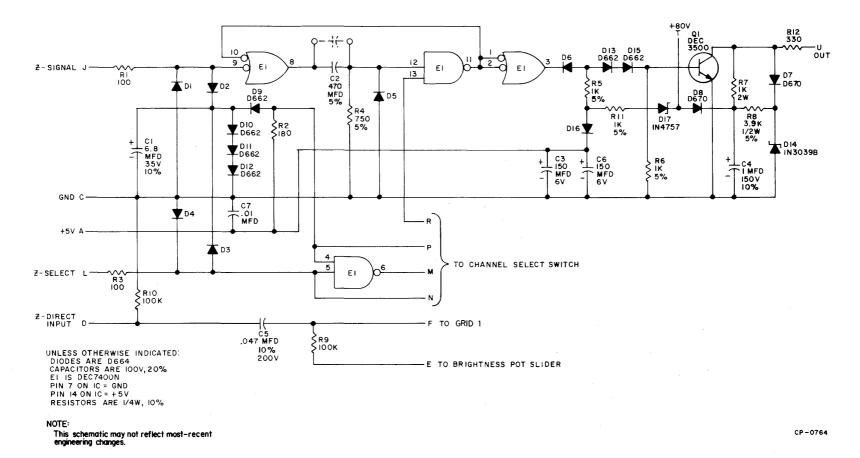
Figure 3-3 Intensity Amplifier W682, Circuit Schematic
