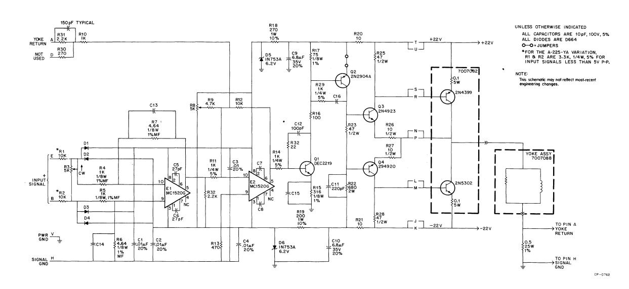
Figure 3-1 X and Y Deflection Circuit
