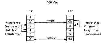
Figure 2-1 Input Power Jumper
