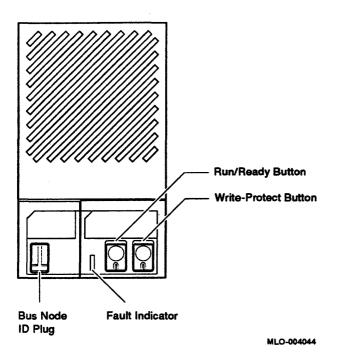
Each ISA has the following controls and indicators on its front panel.
