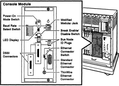
Figure 1–8: Console Module Controls and Connectors
