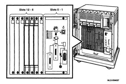
The first four slots are reserved for memory modules. The fifth slot is reserved for the central processing unit (CPU). A console module with system controls and connectors covers these first five slots. Slots 6 through 12 are available for Q-bus option modules.
