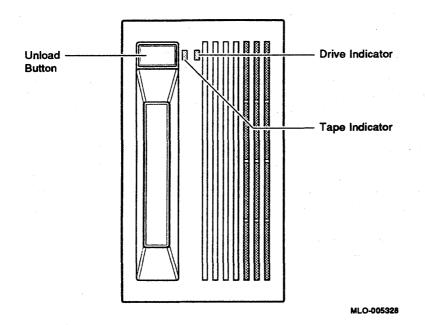
The Unload button is used to eject the cassette tape. The Tape and Drive indicators show the status of the TLZ04 and can indicate possible error conditions.
