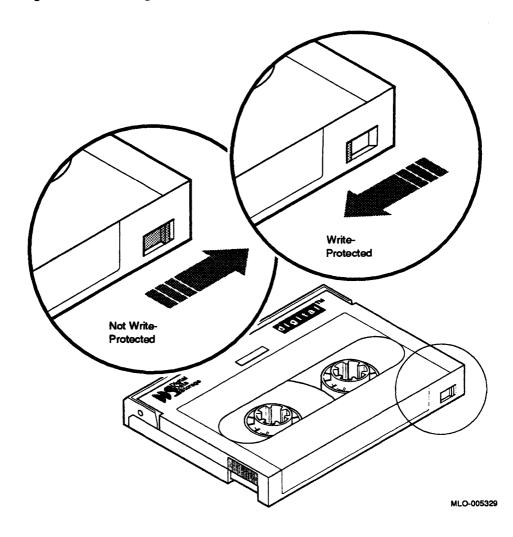
Figure 3-9: Setting the Write-Protect Tab on the Cassette Tape
