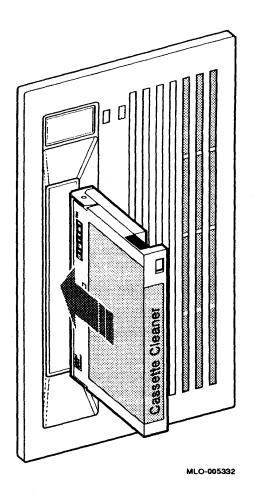
Figure 3–11: Inserting the Head Cleaning Cassette
