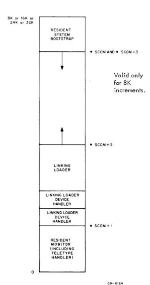
The System Loader learns which I/O handlers are required by the Linking Loader, loads them relocatably, and then loads the Linking Loader relocatably.
