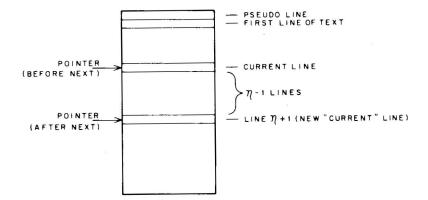
Figure 2-6. Line Buffer After NEXT Command
