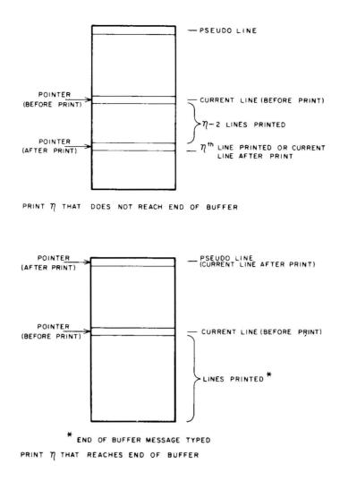
Figure 2-12. Line Buffer After PRINT Command
